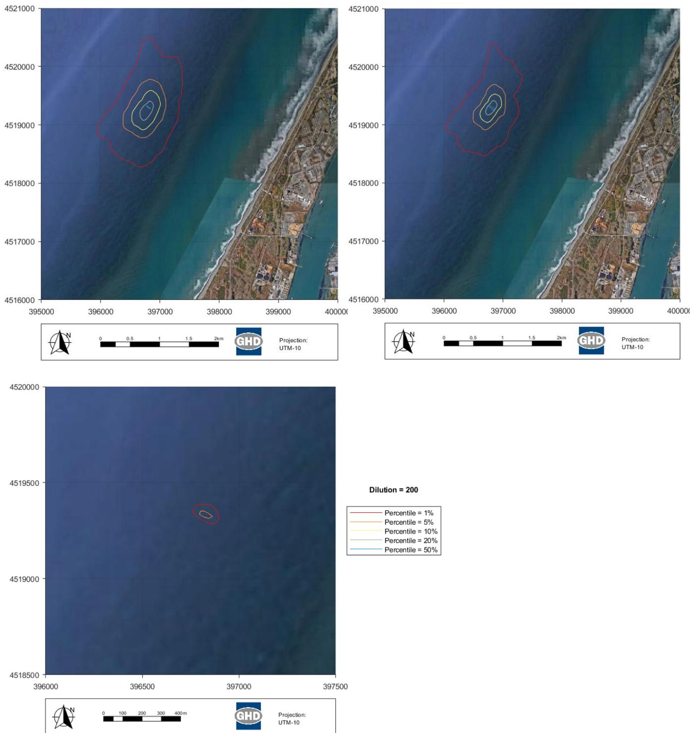
**Image 4-1** Percentile Contours of a Plume Dilution of 200 at the Surface (top left, upper 6.5 feet [2 meters]), Mid-Water (top right, 6.5- 52 feet [2-16 meters]) and Near-Seabed (bottom, > 52 feet [16 meters]) for the Summer Scenario
