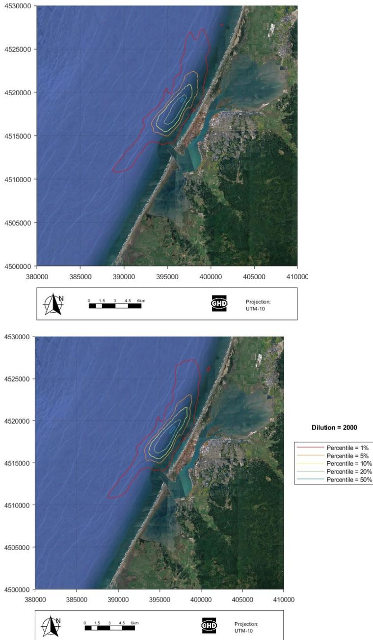
**Image 4-2** Percentile Contours of a Plume Dilution of 2,000 at the Surface (left, upper 6.5 feet [2 meters]) and the Mid- to Lower Portions of the Water Column (right, 6.5-52 feet [2-16 meters]) for the Summer Scenario<sup>2</sup>
