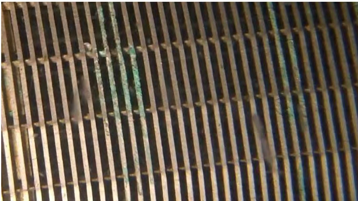
**Figure 5-3.** Video frame grab of the 2 mm screen taken in January 2012 during the wedgewire screen efficiency study with the pump operating. Frame shows an early post-larval fish (est. 16 mm in length) swimming into view above screen (from Tenera 2014b)
