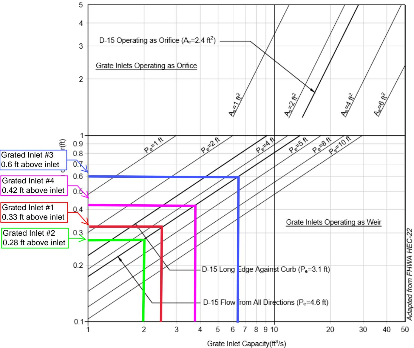
Figure 3-5. Capacity of Grate Inlets in Sag Locations
