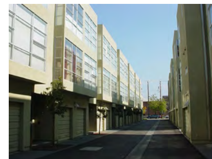
Rear alleys should be used to access residential parking, such as these tuck-under townhouse garages.
