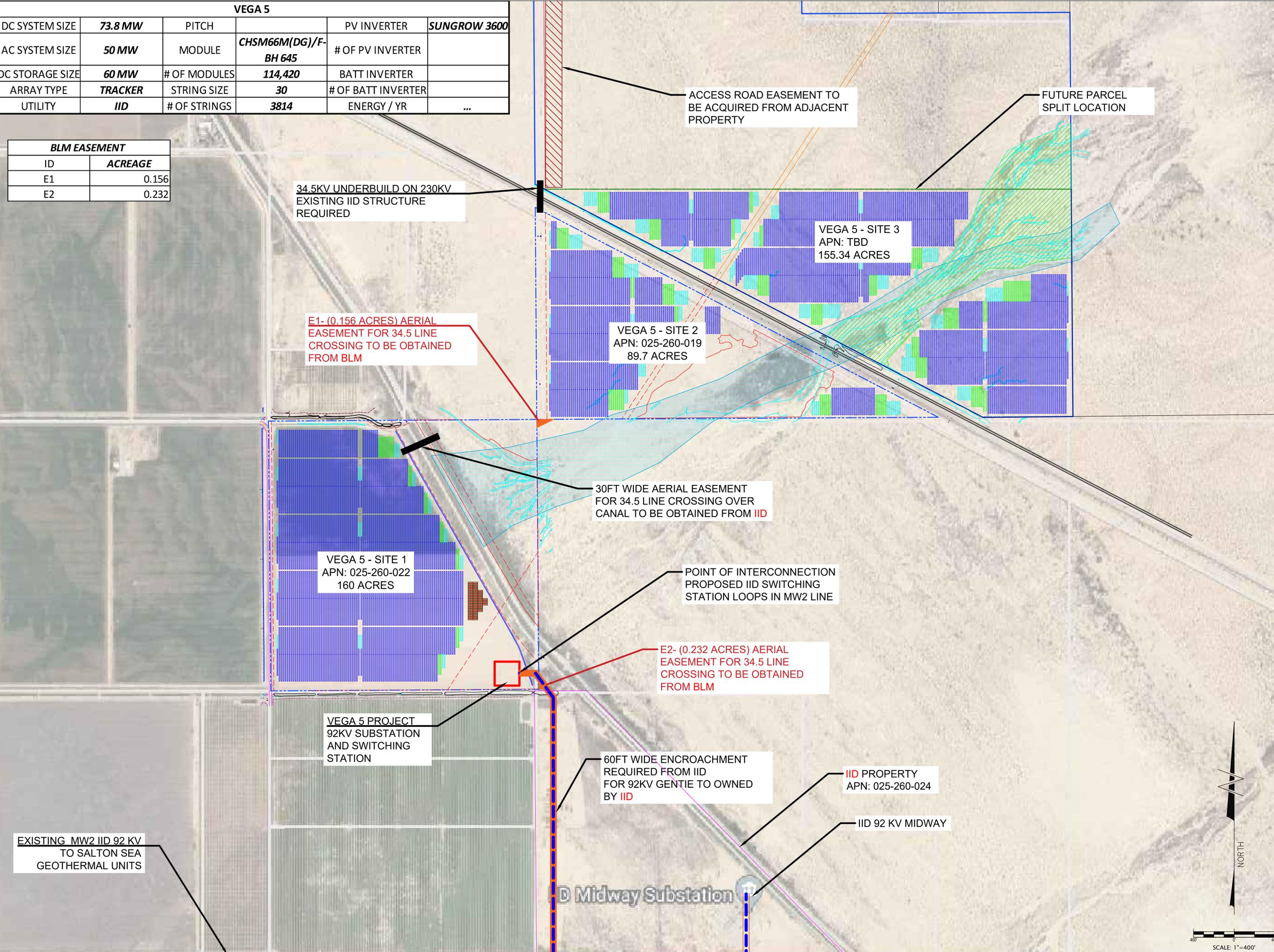
34.5KV UNDERBUILD ON 230KV EXISTING IID STRUCTURE REQUIRED
