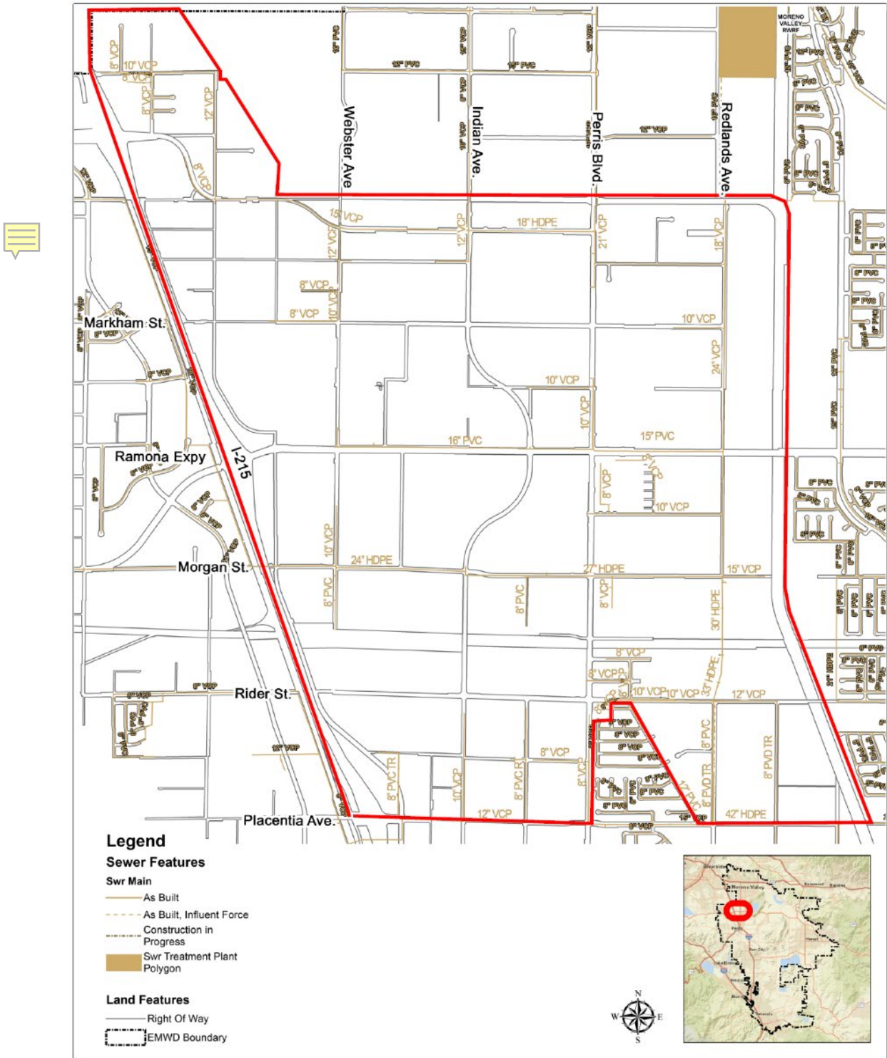
Figure 3.0-8, Existing EMWD Sewer
