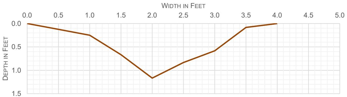
CHART 3. CROSS-SECTION OF DRAINAGE A DOWNSTREAM OF ROAD.
