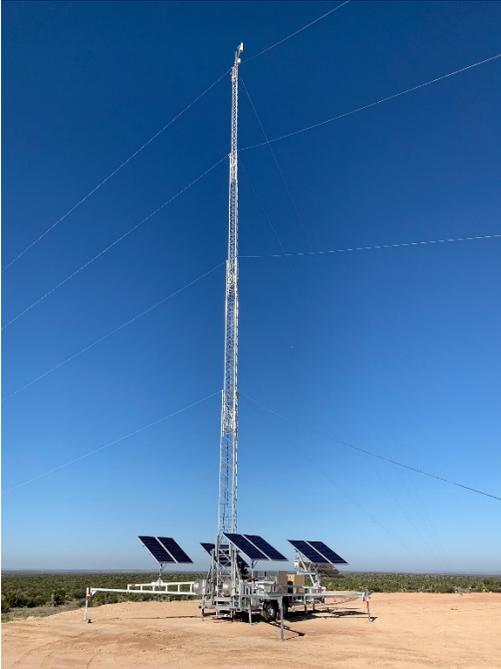
Sample Mid-Deployment Telescoping Lattice Tower Set on Center Support Pole
