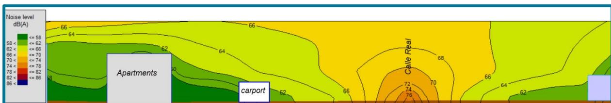
**Figure 6: 3D view of project acoustic model, vertical sound level contours**
