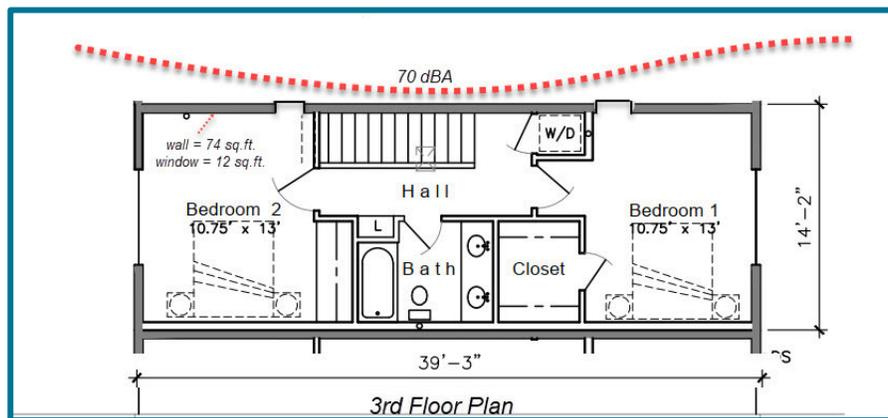
**Figure 8: STC 52 exterior stucco wall, STC 30 window, typical**
