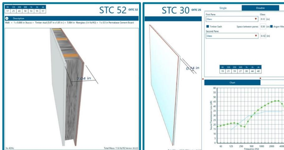
Using these values and making average assumptions for the bedrooms, the predicted interior sound level is found to be 37 dB, which is well within the required annual CNEL 45 dBA required by the California Building Code. See Figure 10 for interior sound level calculation.
