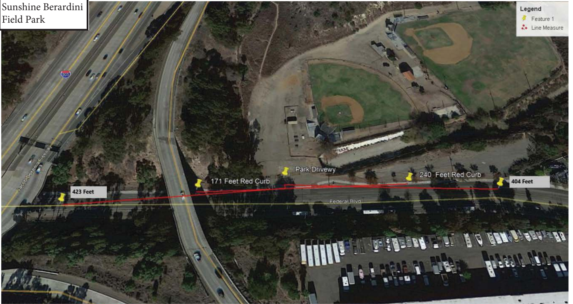
FIGURE 4 - CORNER SIGHT DISTANCE AND RED CURB FOR THE SUNSHINE BERARDINI FIELD PARK DRIVEWAY
