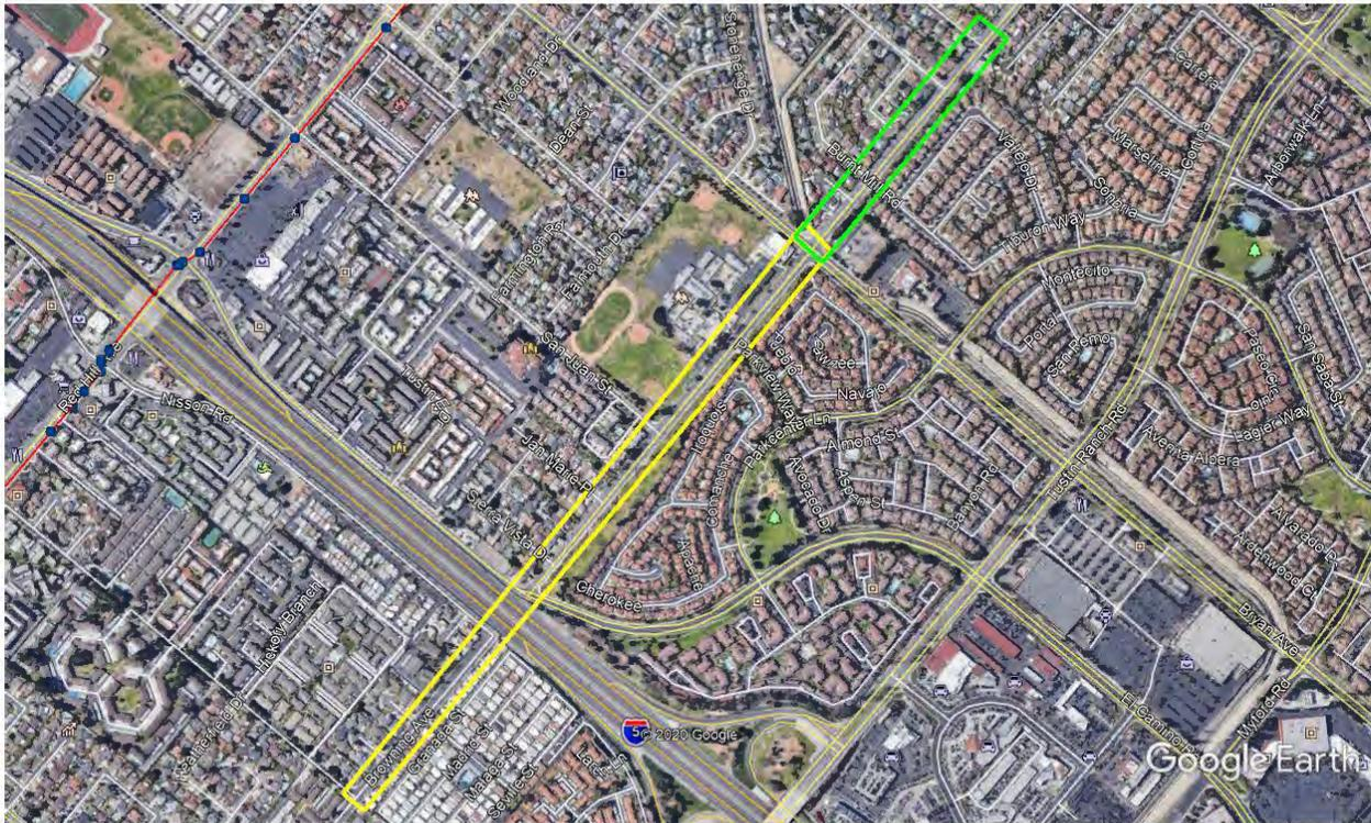
Segment 2 – This segment will replace and upsize 2,475 feet of 12-inch sewer in Browning Road between Bryan Avenue and the I-5 Freeway and upsize of approximately 1,500 feet of 10-inch sewer between Bryan Avenue and Bent Twig Lane. The recommended replacement sizes are 18-inches (replacing the 12-inch pipes) and 15-inches (replacing the 10-inch pipes.)
