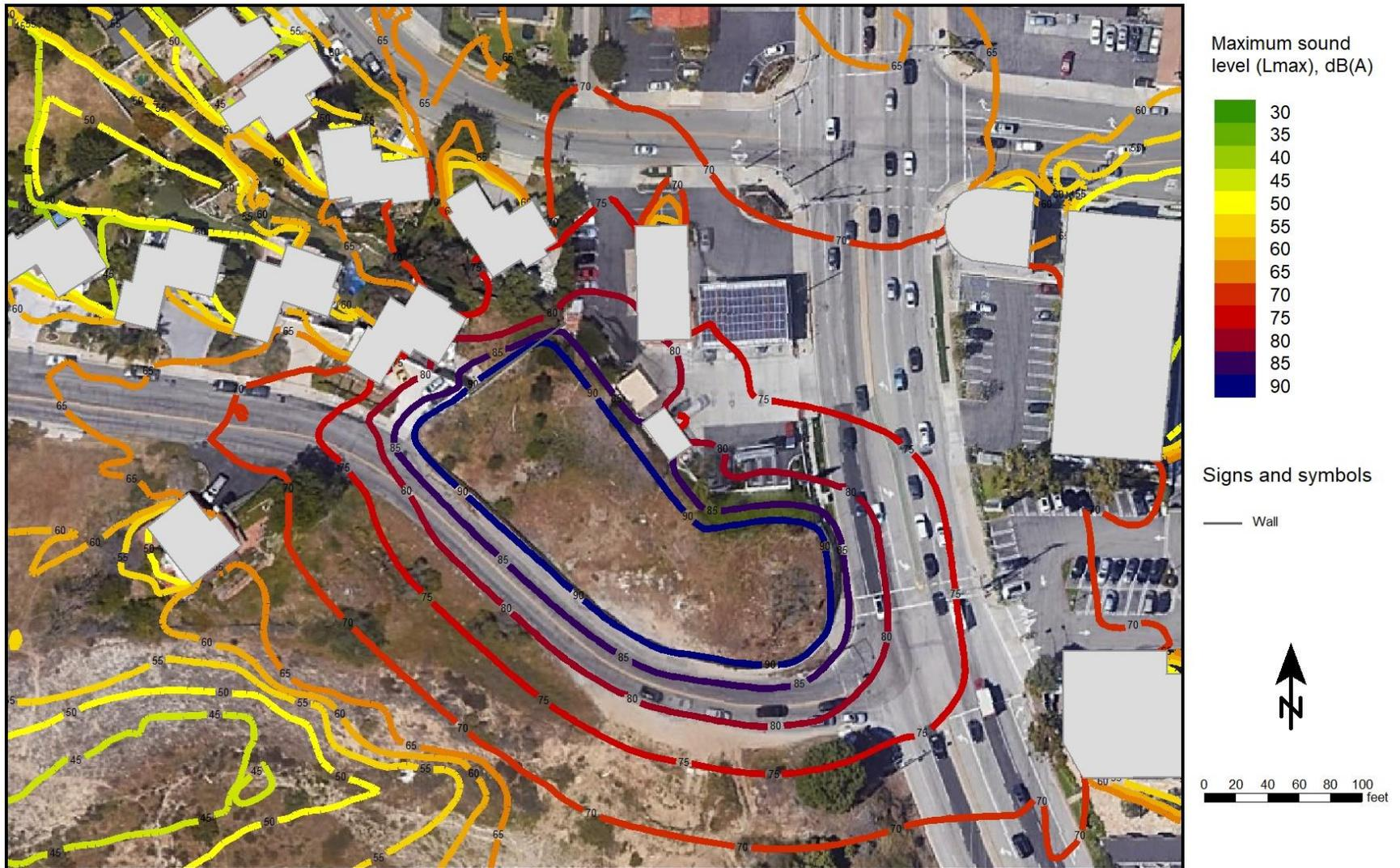
Figure 6 Unmitigated excavation phase noise contour map
