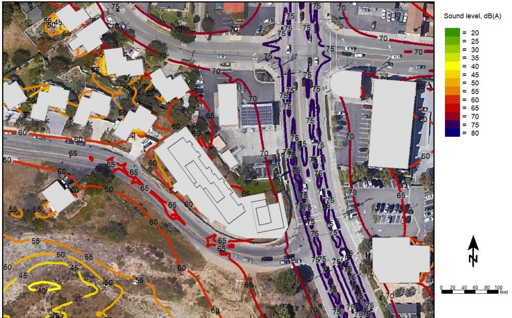
Figure 4 Predicted Future CNEL Noise Levels 5 ft Above Ground Level (First Floor Locations)
