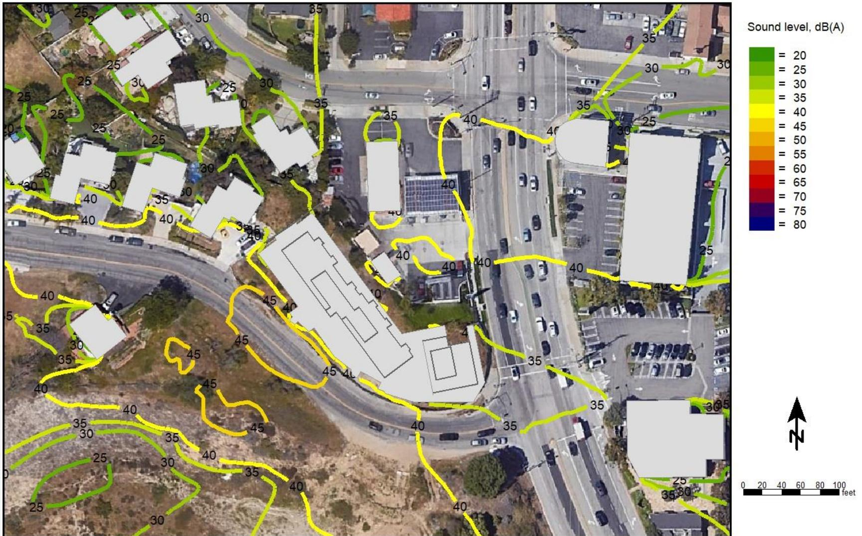
Figure 3 Roof top air conditioning unit operational noise level contour map
