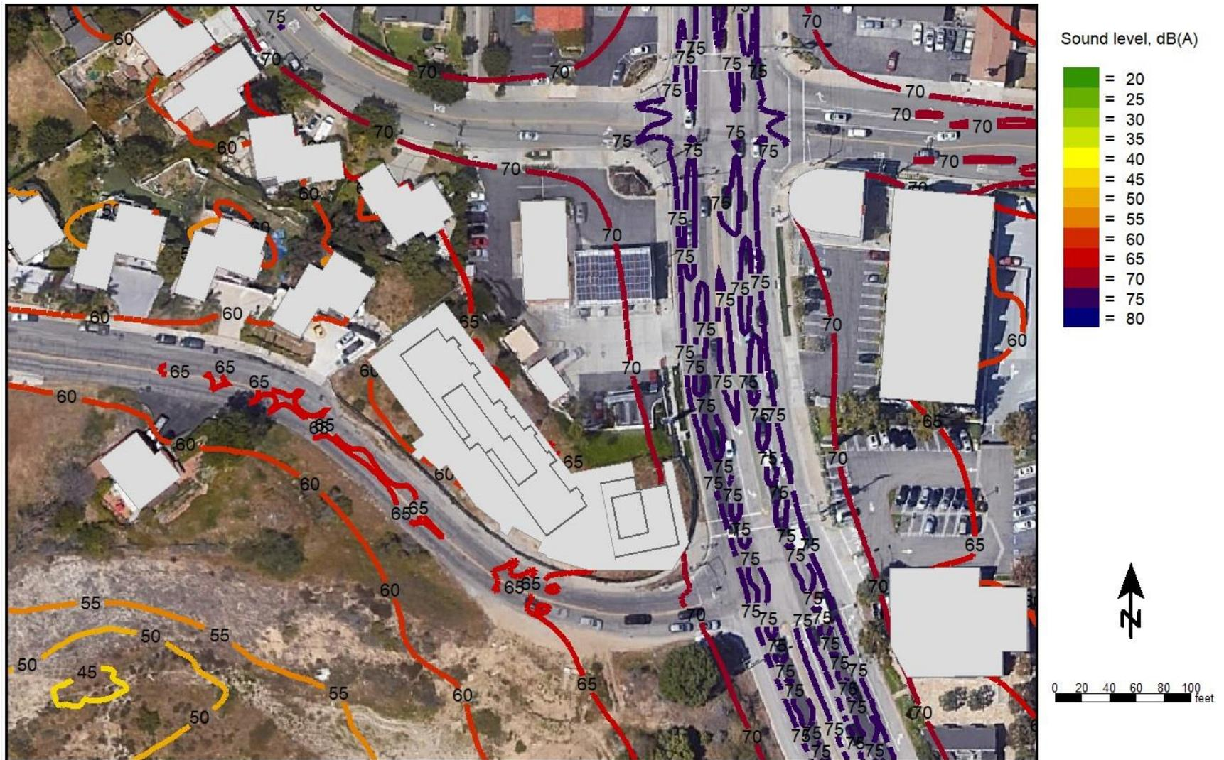
Figure 5 Predicted Future CNEL Noise Levels 8 ft Above Ground Level (Second Floor Locations)
