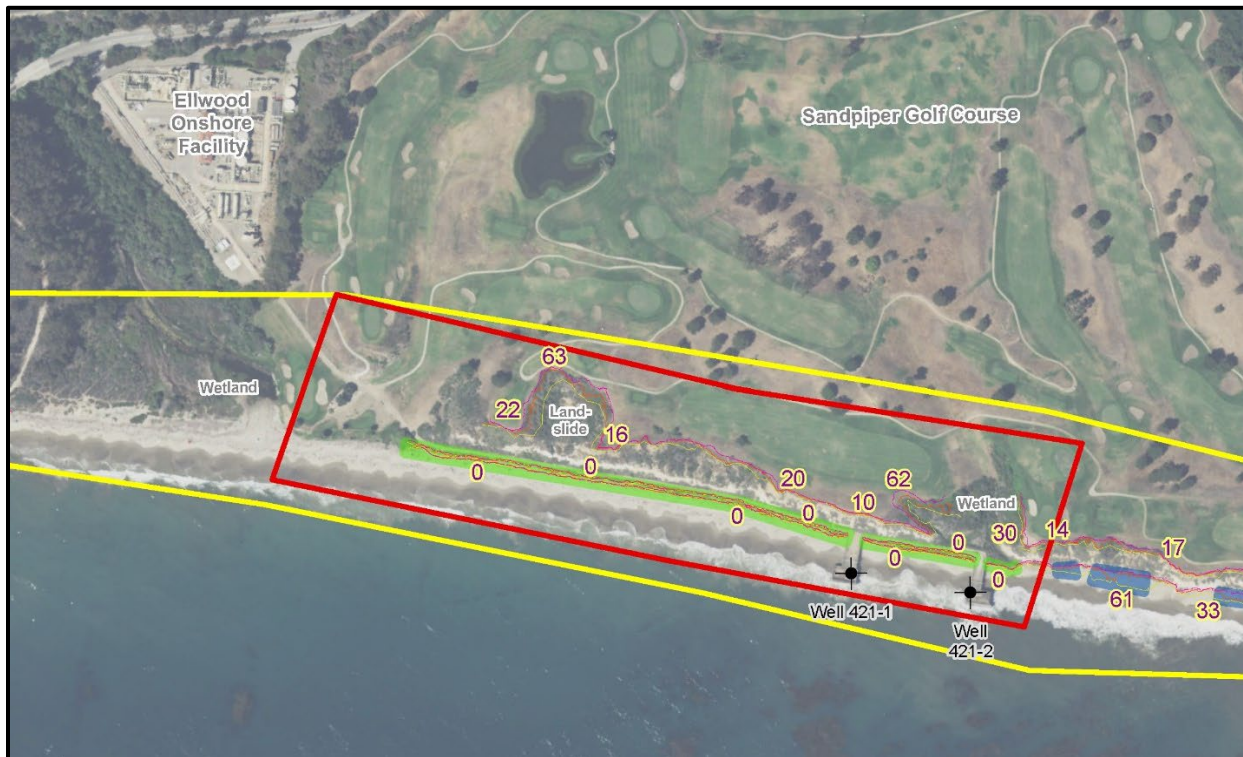
Figure 4.6-3. Bluff Retreat Rates in the Project Area (centimeters per year) (Excerpt from Plate 5 of Appendix G)
