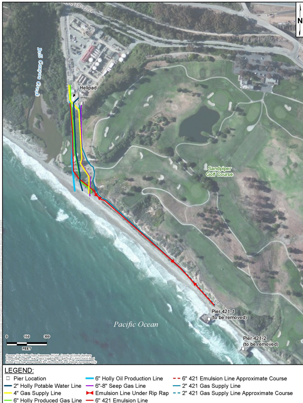
Figure 2-17. Pipelines from the EOF to the 421-1 and 421-2 Piers
