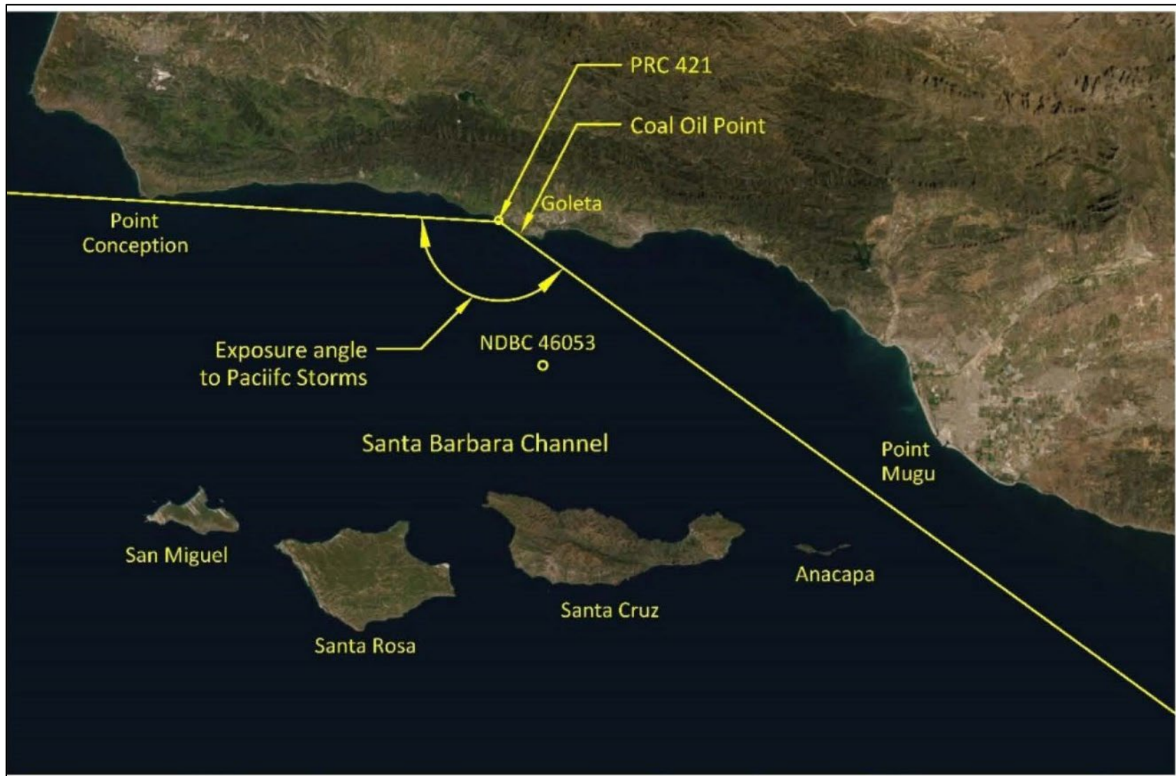
Figure 8-1. PRC 421 Exposure Angle to Pacific Storms
