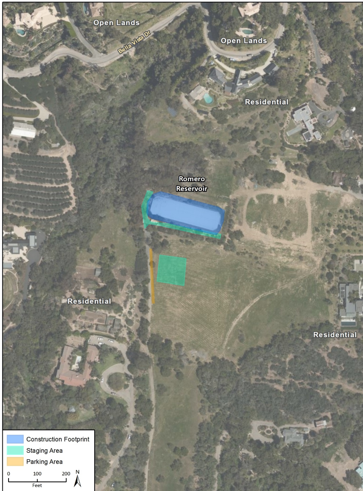
Figure 5 Romero Reservoir Construction, Staging, and Parking Areas
