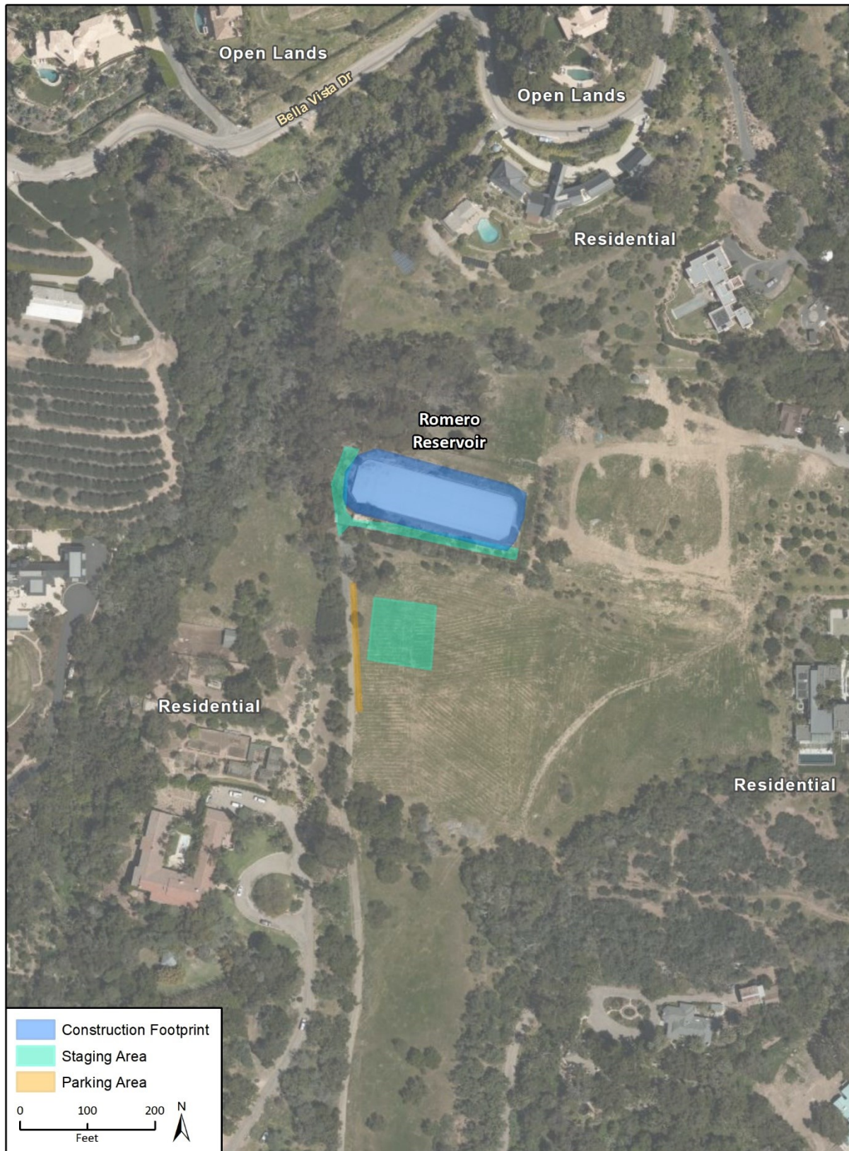
Figure 3 Romero Reservoir Construction, Staging, and Parking Areas
