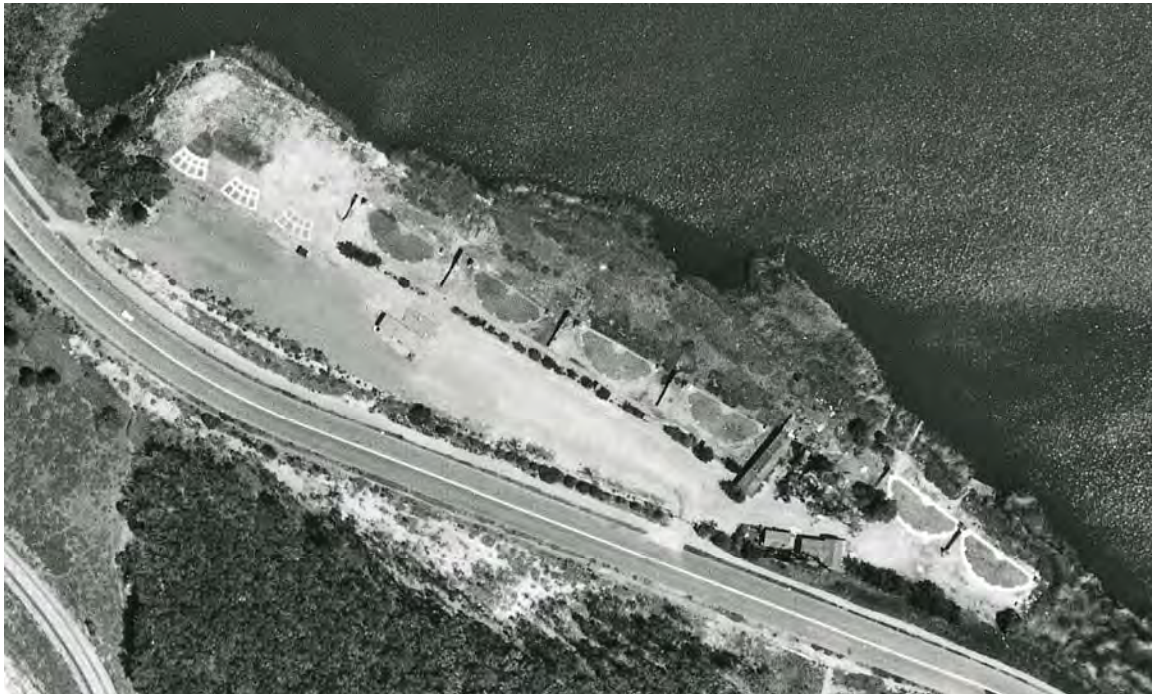
Historic Image 14. Aerial view in 1955. Changes since 1950 aerial (Historic Image 13) include completion of trap field complex (Fields 1 to 3), addition of concrete skeet station path around Fields 4 to 7 on western end of site, and construction of skeet fields (Fields 8 and 9) at eastern end of site. Source: Pacific Aerial Surveys.
