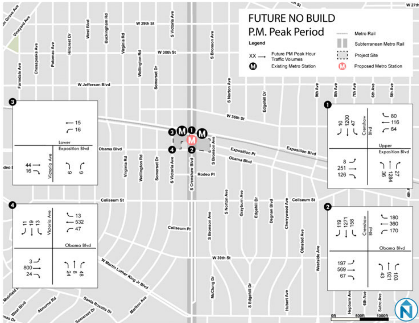
Figure 17 Future (2023) No Project Turning Movements (PM Peak)
