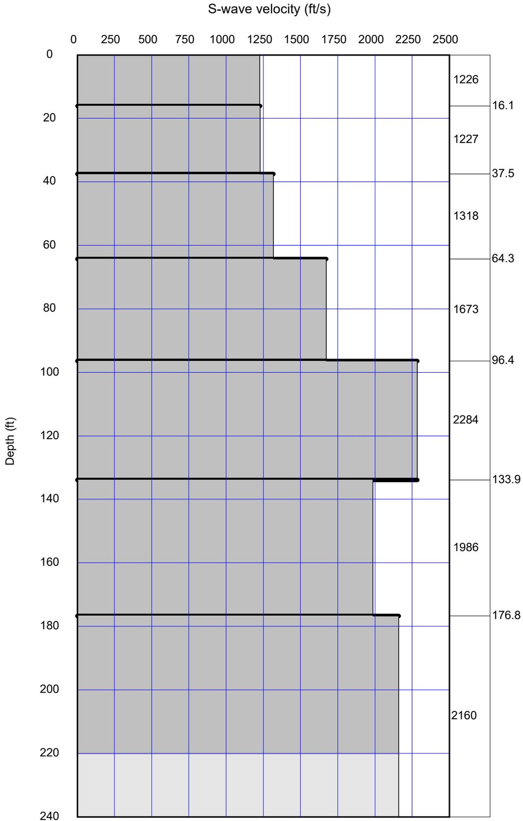
S-wave velocity model (inverted) : Final.rst **Average Vs 100ft = 1395.7 ft/sec**
