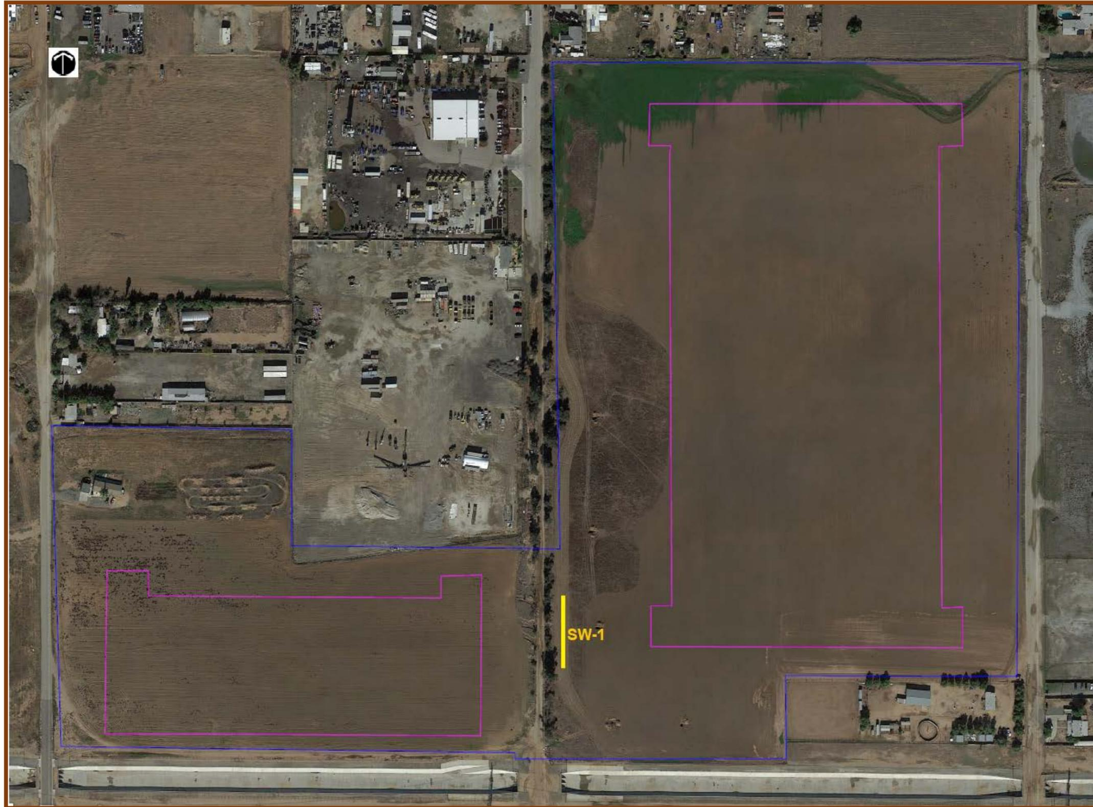
Base Map: Provided by client; Seismic shear-wave survey line (SW-1) shown as yellow line, proposed buildings outlined in purple.
