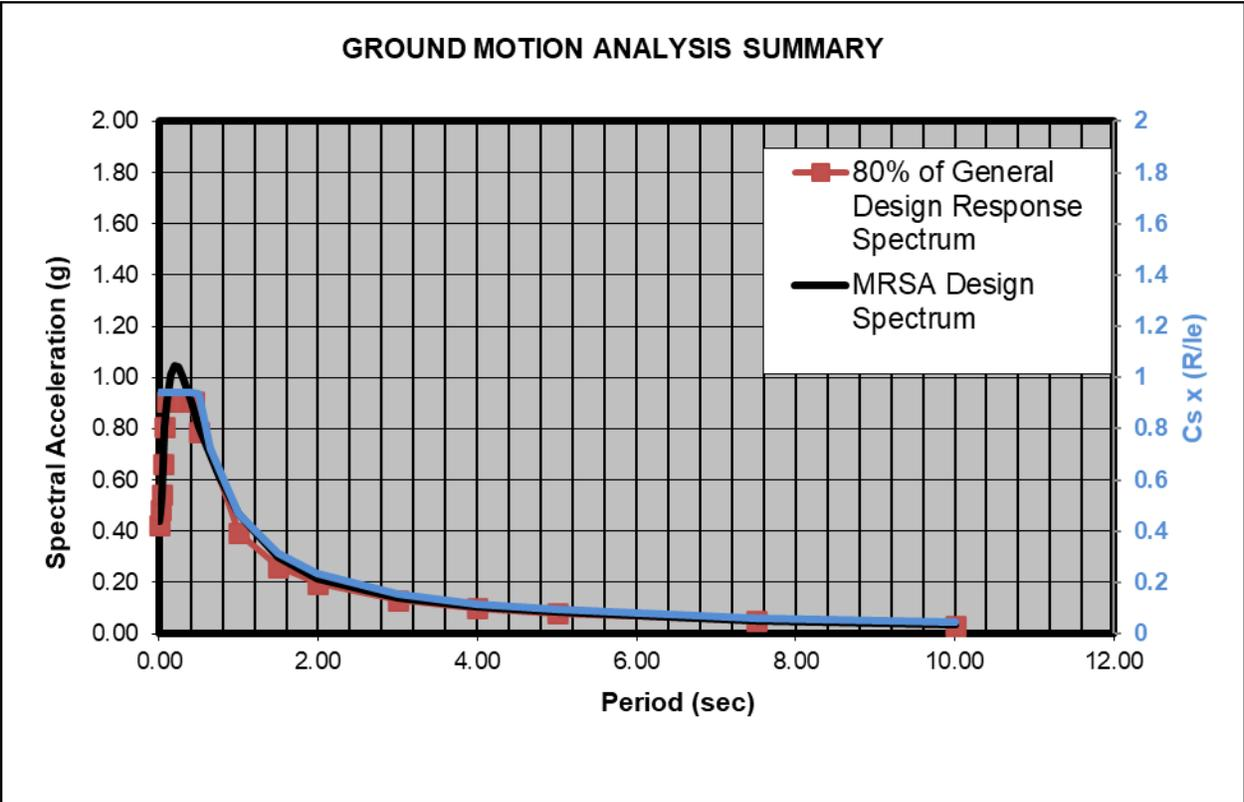
◆ **Design Acceleration Parameters (ASCE 7 Section 21.4)-**
