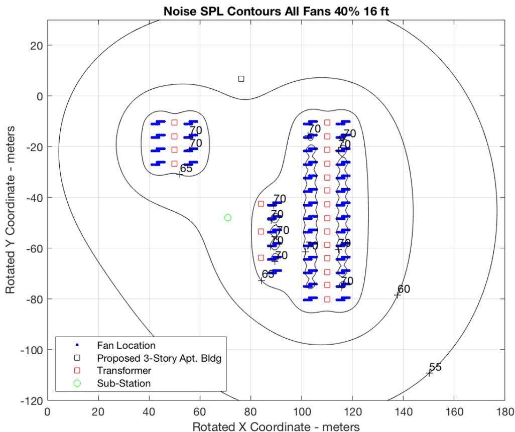
Figure 10. Fans Only Noise Sound Level Contours at 16 ft Elevation with All Fans Running at 40%
