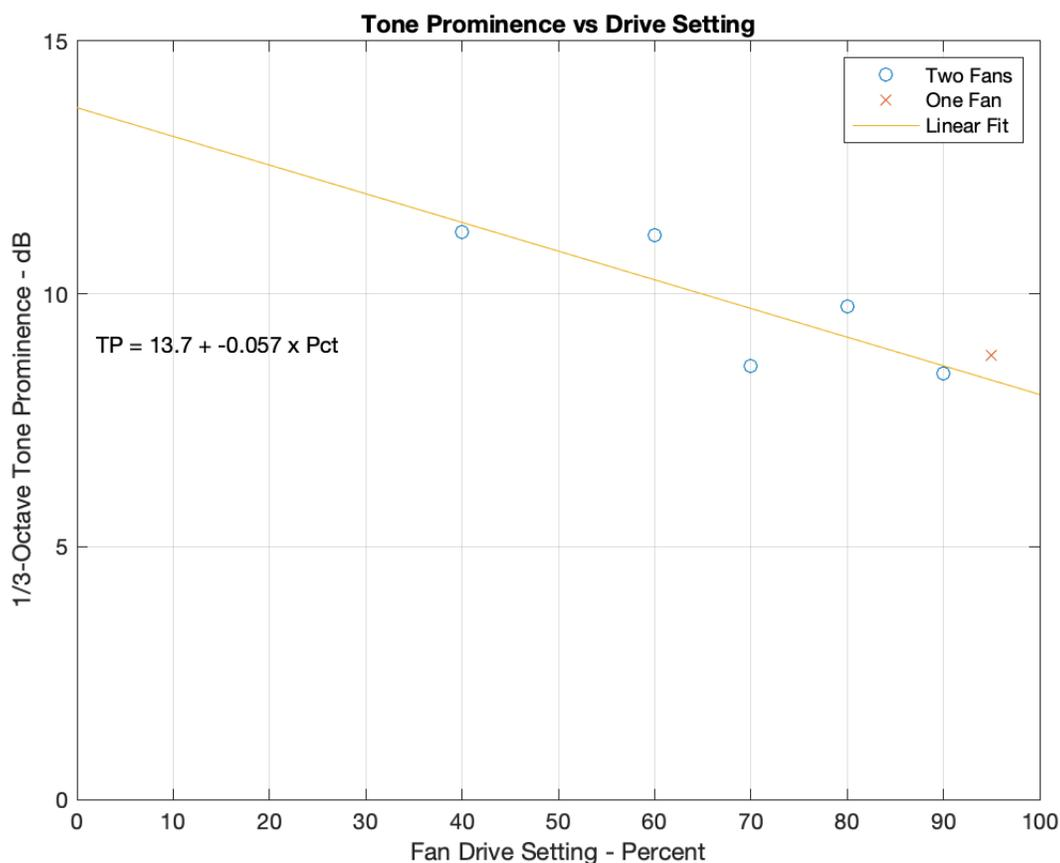
Figure 8. Tesla Cooling Fans Blade Passage Tone Prominence vs Drive Setting
