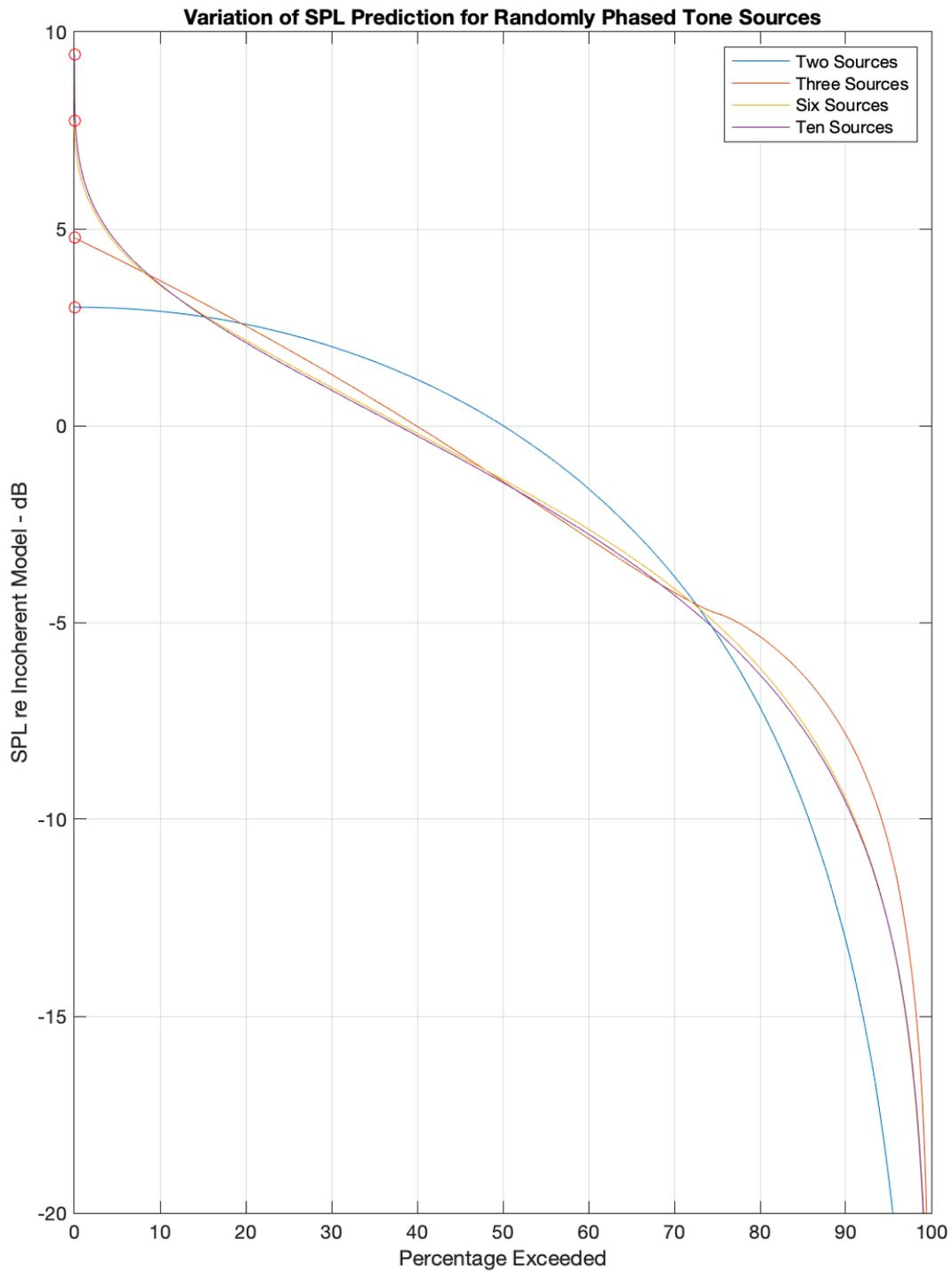
Figure 9. Summing Two, Three, Six or Ten Equal Tonal Sources with Random Phases
