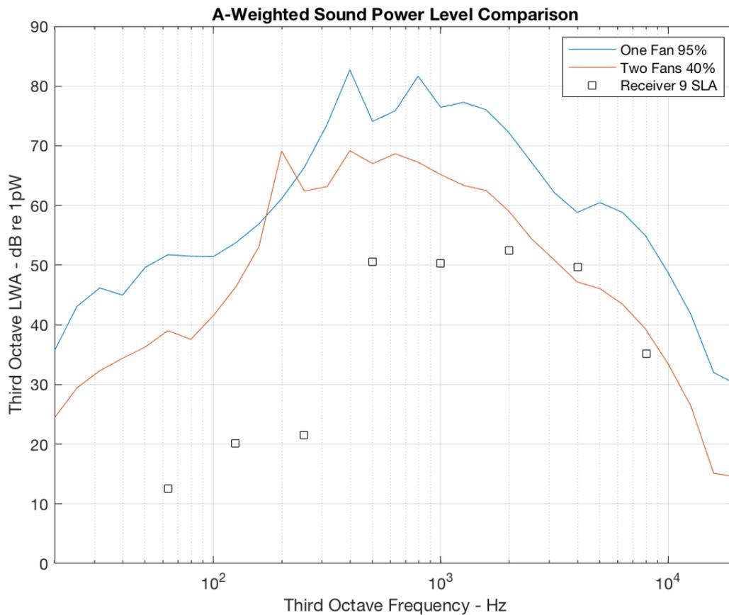
Figure 7. Third-Octave A-Weighted Sound Power Level Spectra (Receiver 9-3 is Octave Band SLA in dB re 20  $\mu$ Pa)
