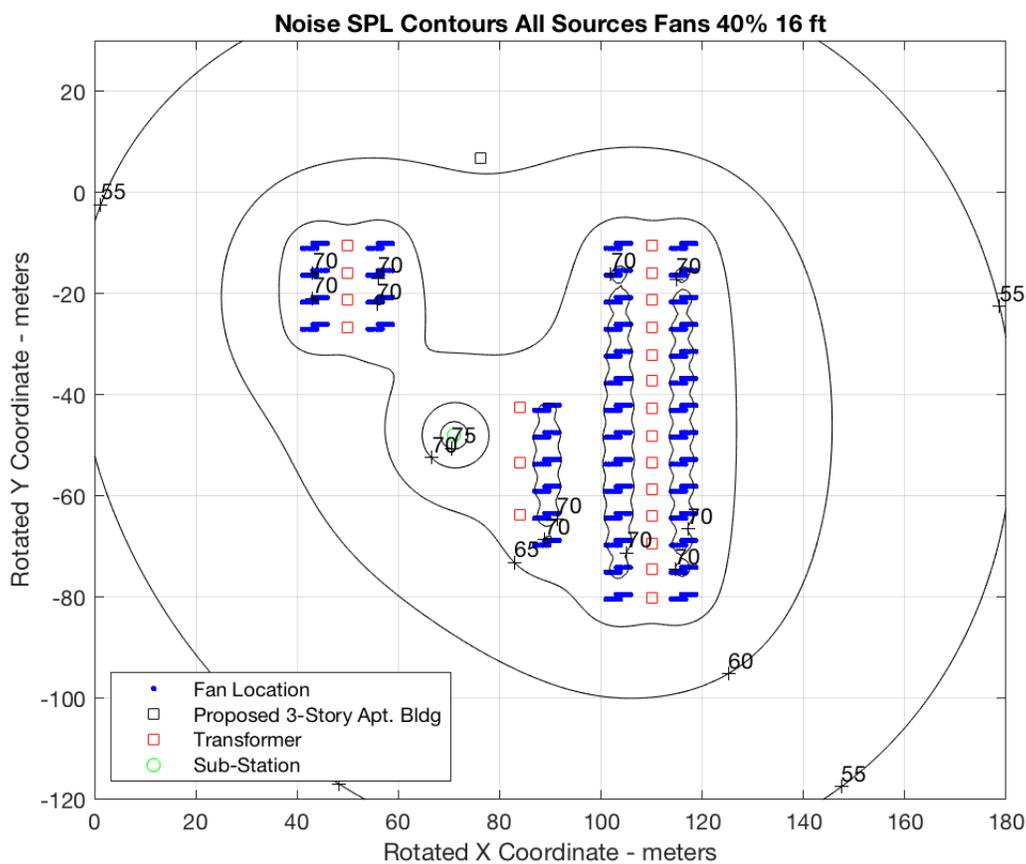
Figure 11. Approximate (unshielded) Noise Contours for All Fans, Transformers and Sub-Station
