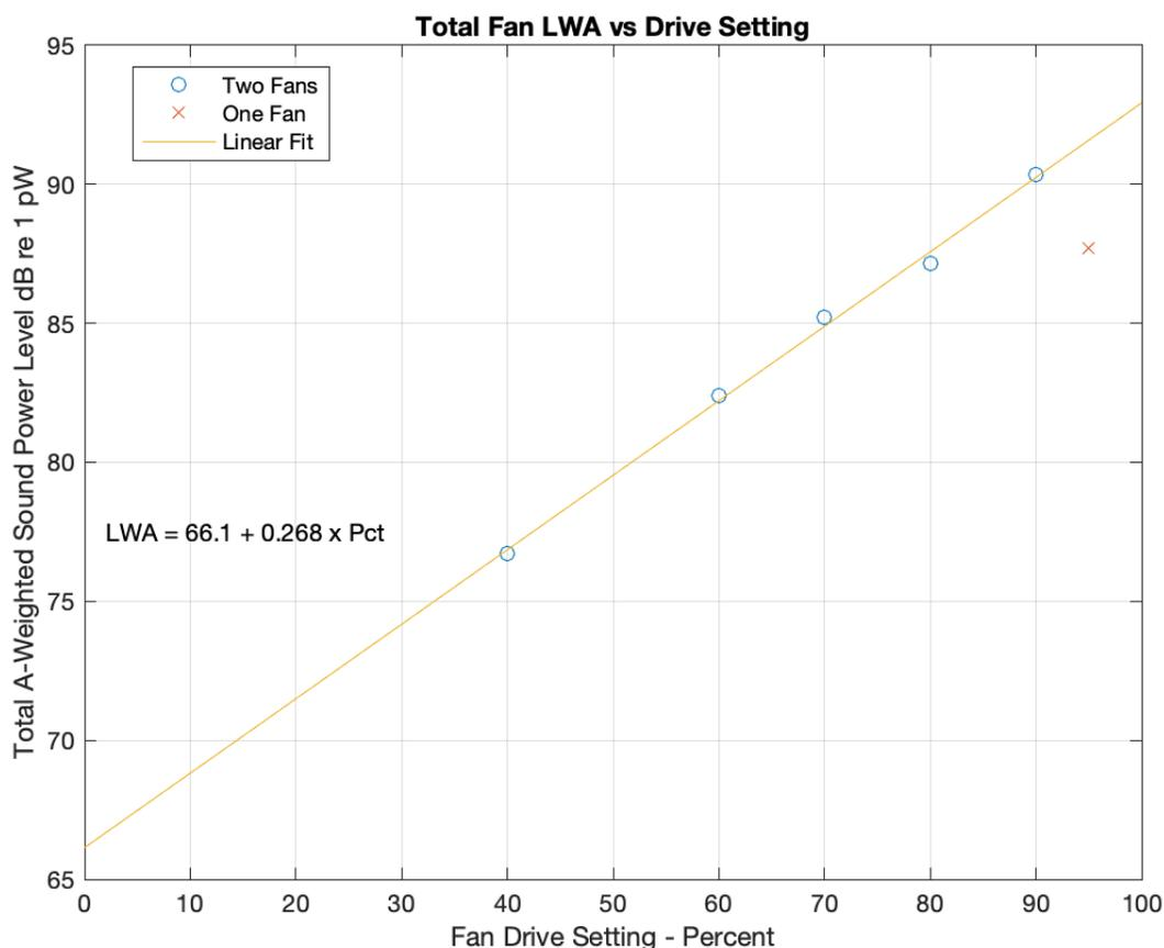
Figure 6. Tesla Cooling Fans Total Sound Power Level vs Drive Setting
