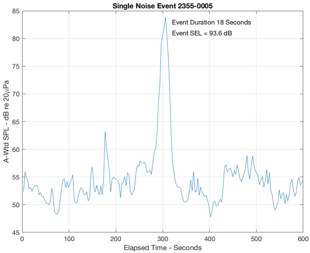
Figure 4. Detail of Midnight Noise Event from Long Term Measurement Data
