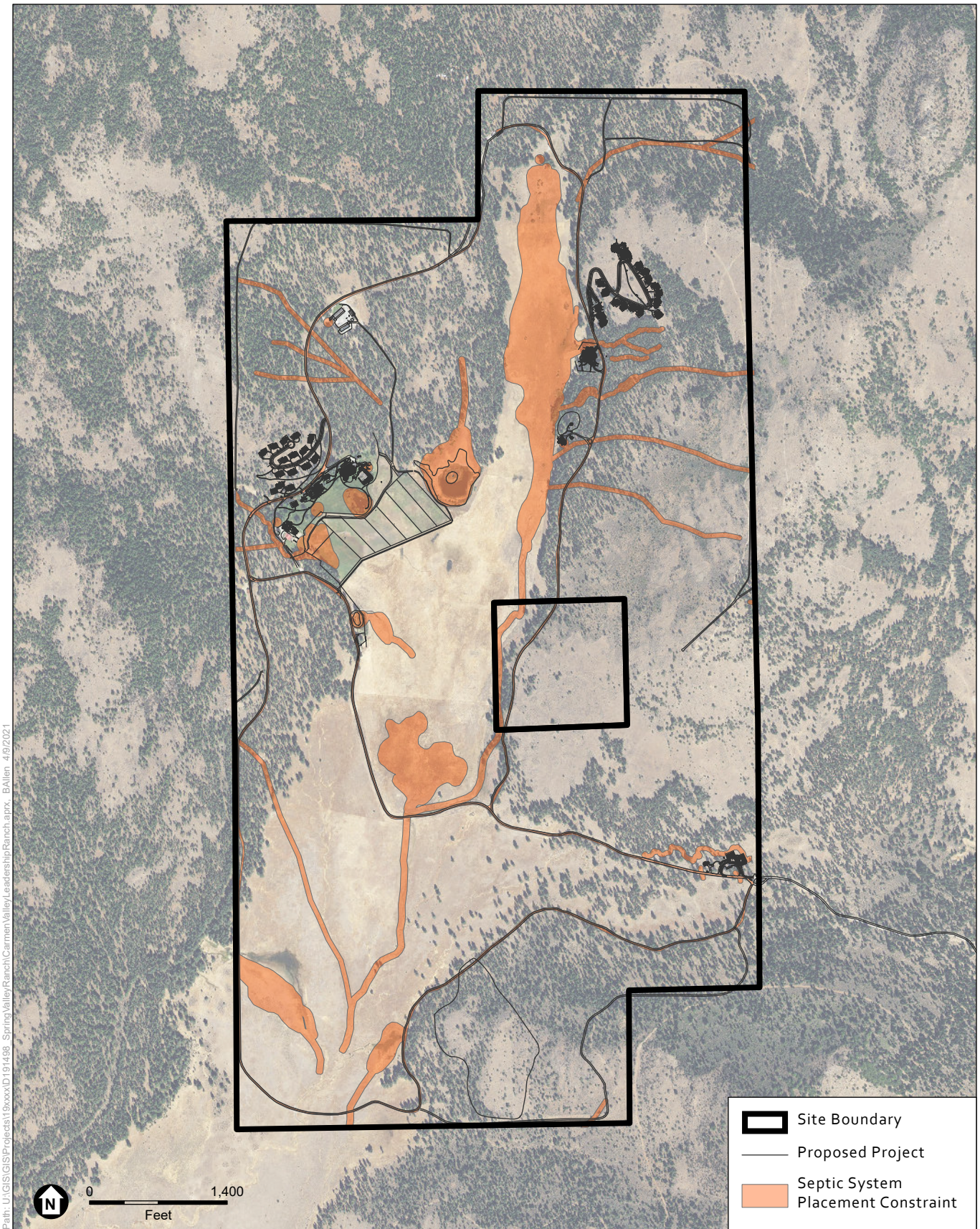
Figure 10 Septic System Placement Considerations
