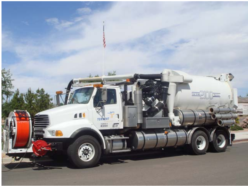
Typical Hydrovactor Truck used for Drywell Maintenance
