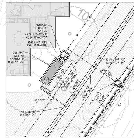
**STORMWATER QUALITY (MWS-A1) TYPICAL DIVERSION SCHEMATIC**
