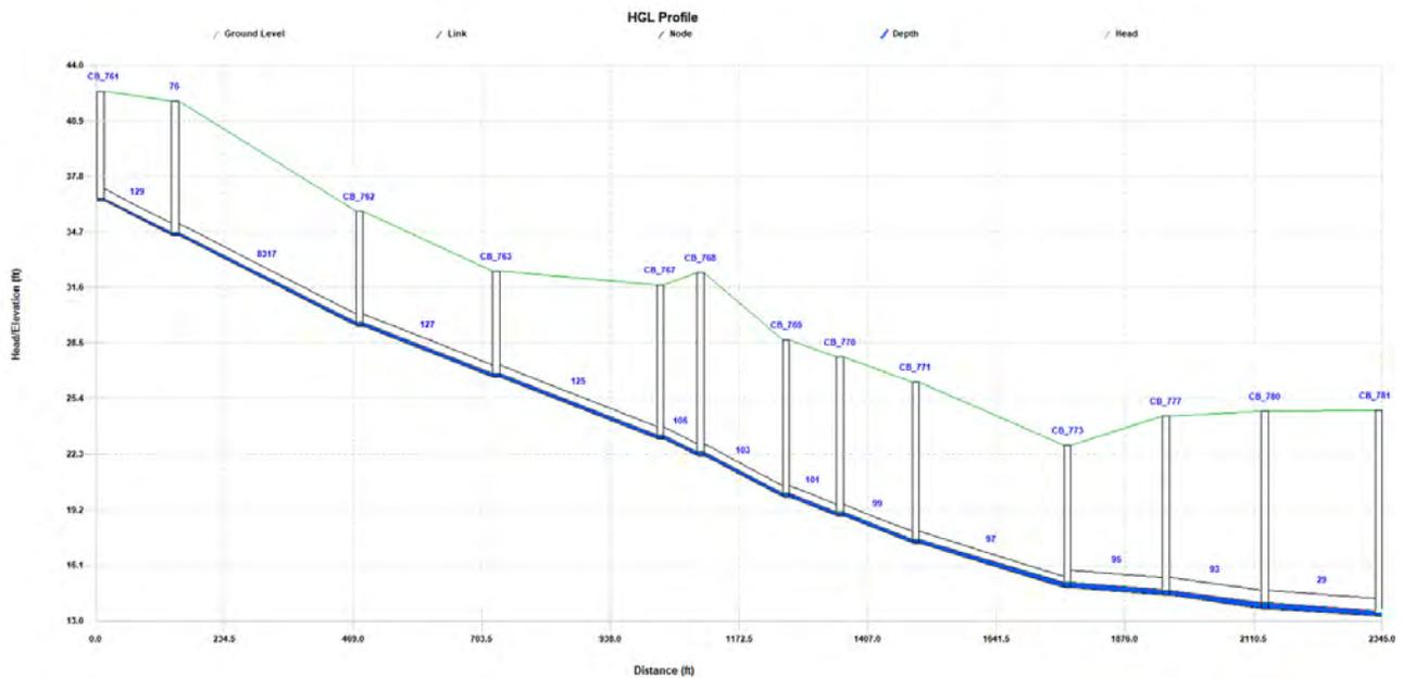
Per the “Conceptual Utility” drawing provided by SCWD (Appendix B), the Project’s sewage will flow to the existing 8-inch sewer in Sepulveda Ave.
