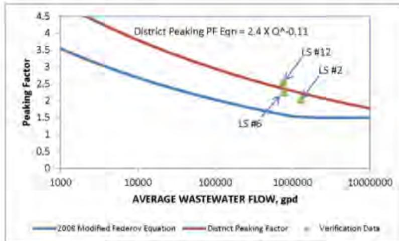
**Figure 5-12 Sewer System Peaking Factors**
