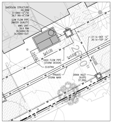
**STORMWATER QUALITY (MWS-A4) TYPICAL DIVERSION SCHEMATIC**
