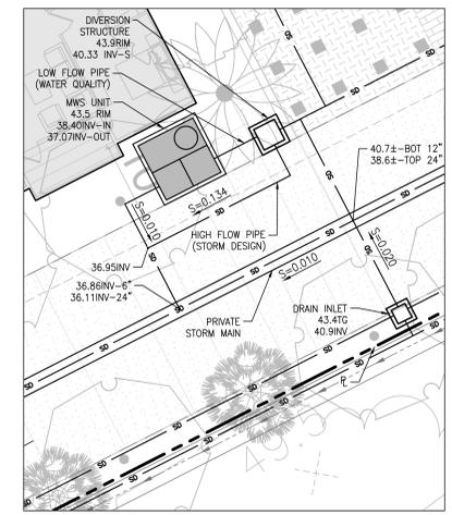
**STORMWATER QUALITY (MWS-A2) TYPICAL DIVERSION SCHEMATIC**
