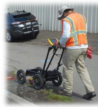
GPR Data Collection
