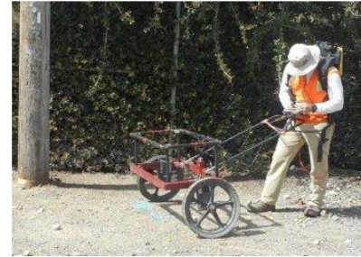
EM-61 data acquisition
