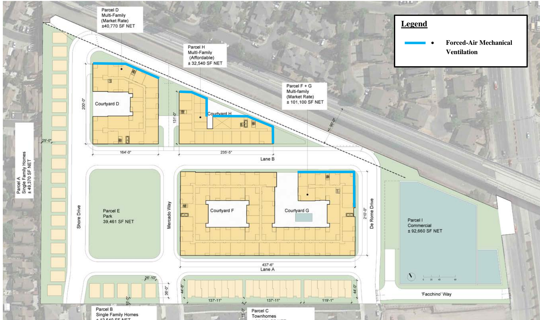
FIGURE 5 Locations Where Noise Abatement Measures are Recommended
