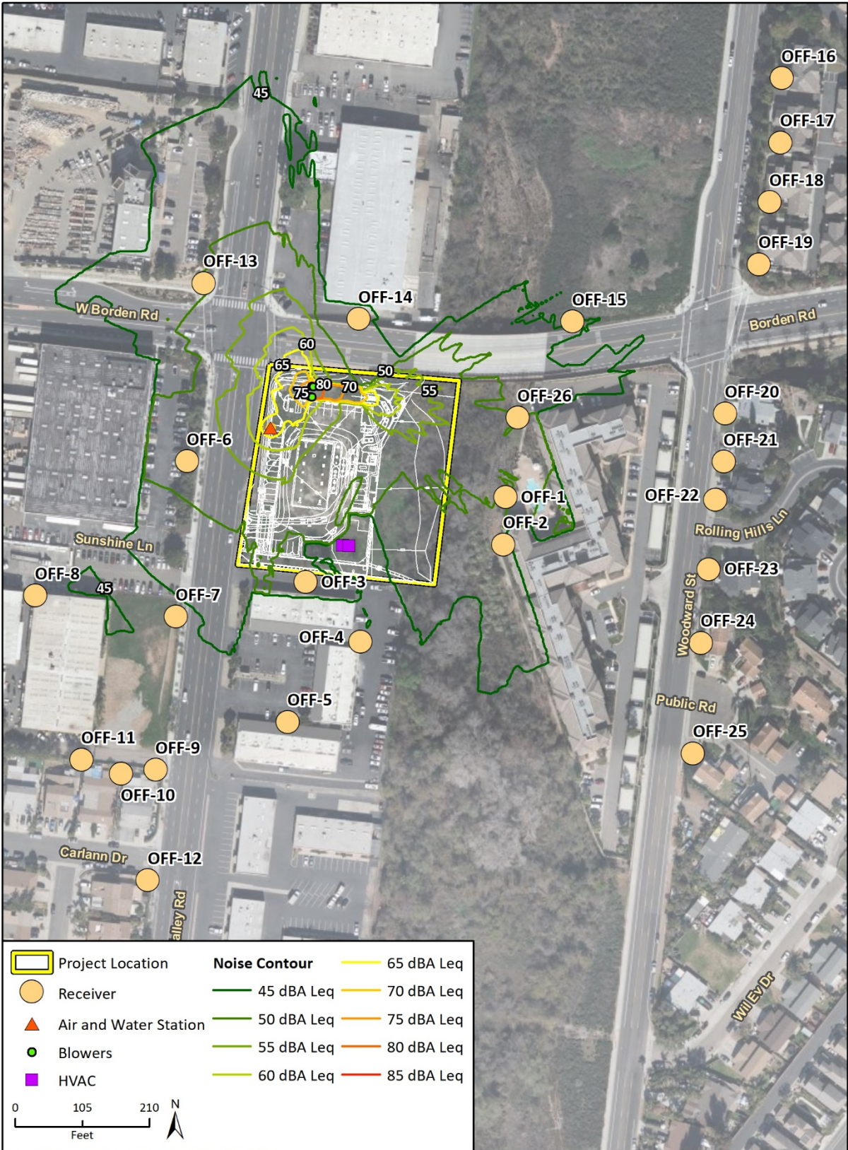
Figure 4 Off-site Receivers and Daytime Operational Noise Contours
