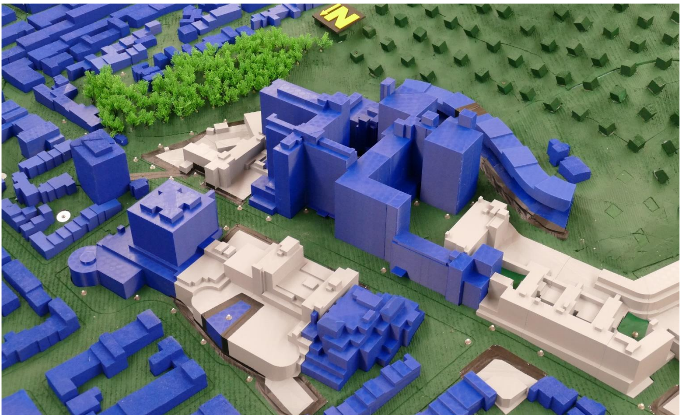
Figure 1A: Photographs of Wind Tunnel Test Model – Existing
