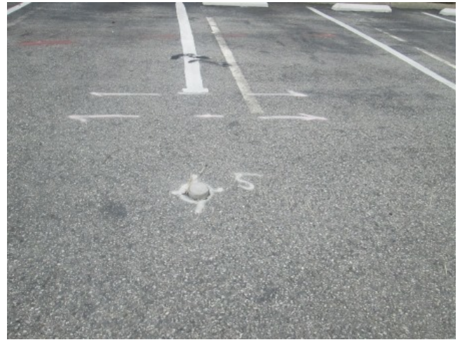
Evidence of former soil boring on north- northwest exterior of 577 Building
