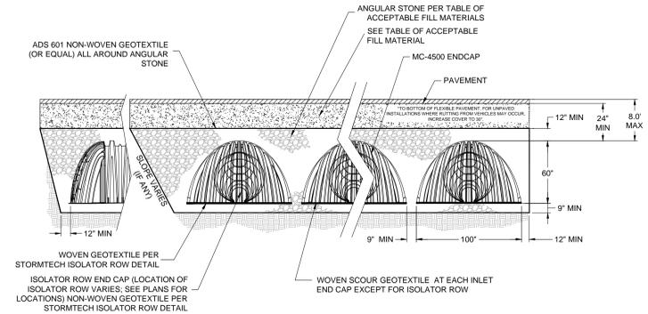
THE INSTALLED CHAMBER SYSTEM SHALL PROVIDE THE LOAD FACTORS SPECIFIED IN THE AASHTO LRFD BRIDGE DESIGN SPECIFICATIONS SECTION 12.12 FOR EARTH AND LIVE LOADS, WITH CONSIDERATION FOR IMPACT AND MULTIPLE VEHICLE PRESENCES.
