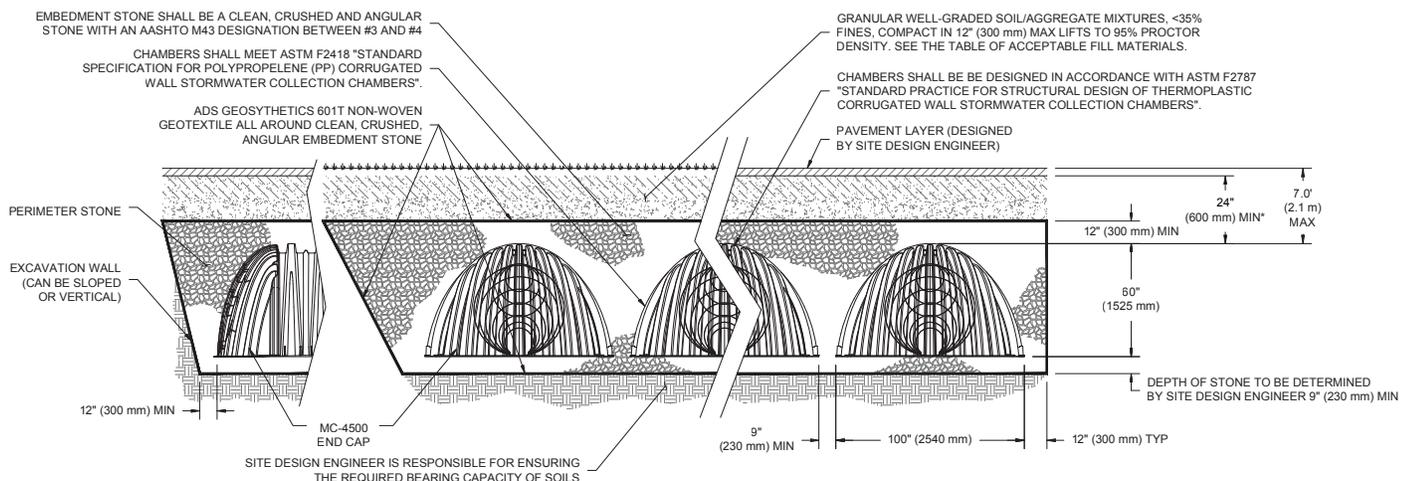
\*MINIMUM COVER TO BOTTOM OF FLEXIBLE PAVEMENT. FOR UNPAVED INSTALLATIONS WHERE RUTTING FROM VEHICLES MAY OCCUR, INCREASE COVER TO 30" (750 mm).
