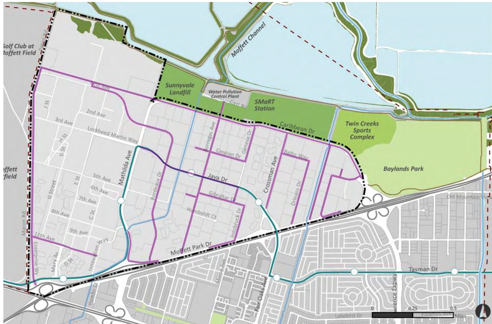
FIGURE 64 Existing Recycled Water System
