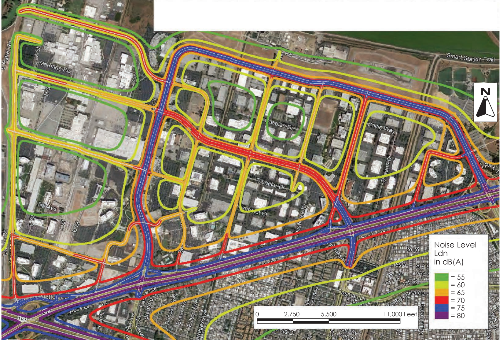
CUMULATIVE PLUS PROJECT 2040 TRAFFIC NOISE CONTOURS
