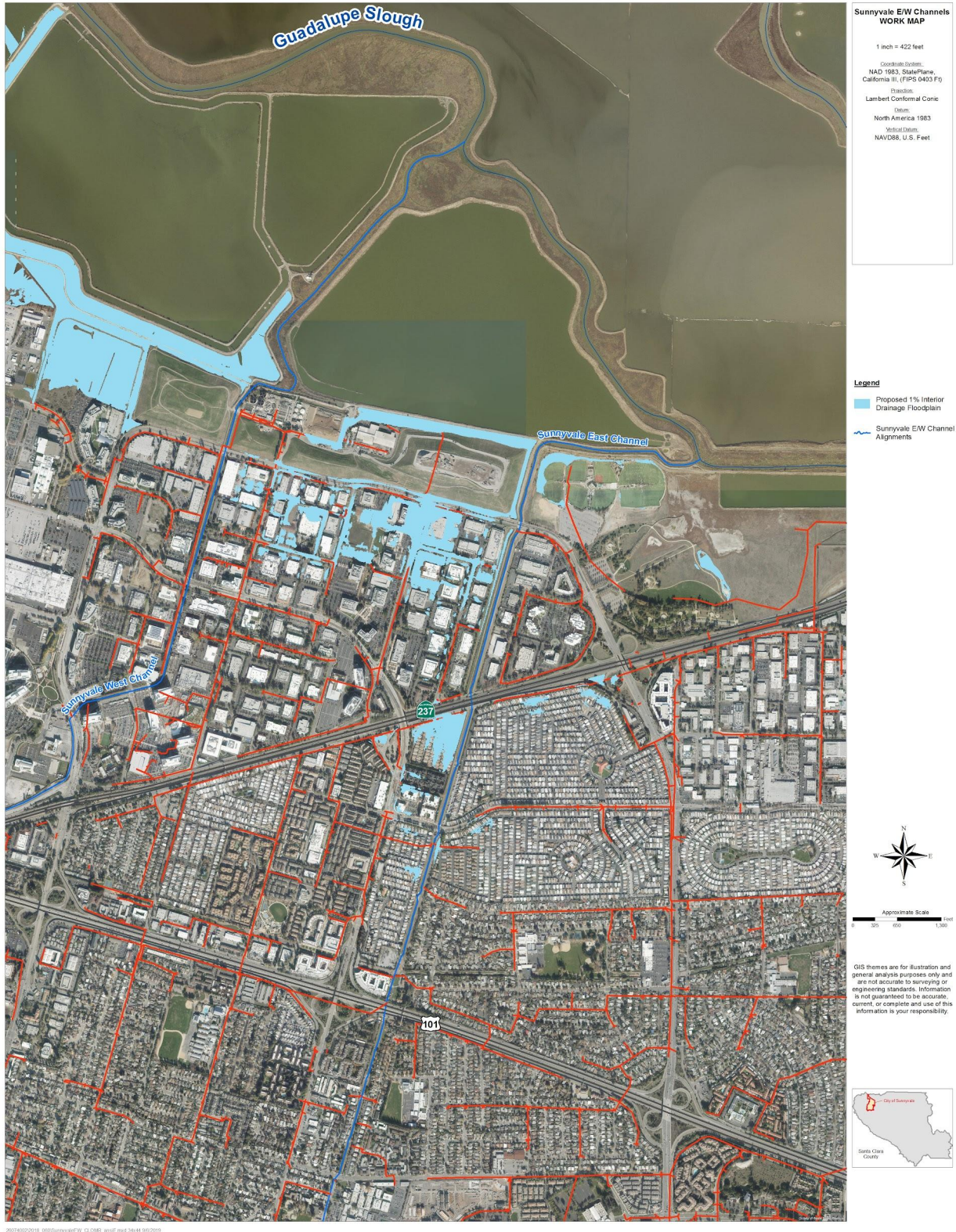
Figure 3. Residual flood risk in Moffett Park after construction of a shoreline flood risk management levee and completion of Sunnyvale East and West channel upgrades.
