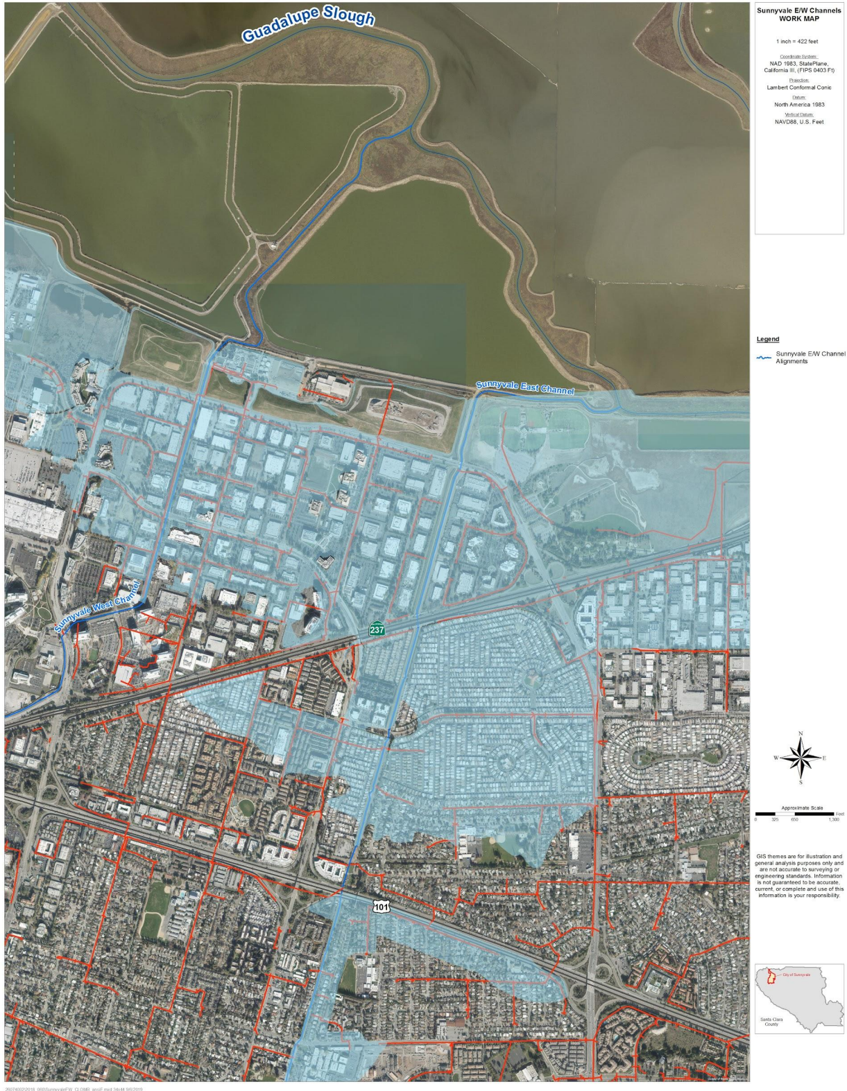
Figure 2. The existing flood risk areas for a 1% flood event from FEMA's effective map, including riverine, interior, and coastal flood risks (assume levee failure).
