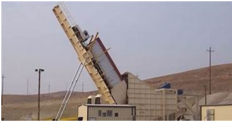
Exhibit 2 Example Hydraulic Truck Dump
