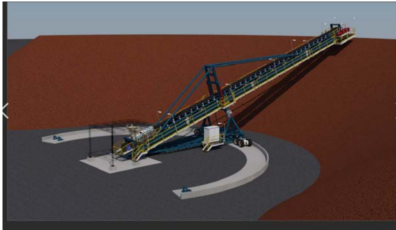
Exhibit 3 Example Radial Stacker
