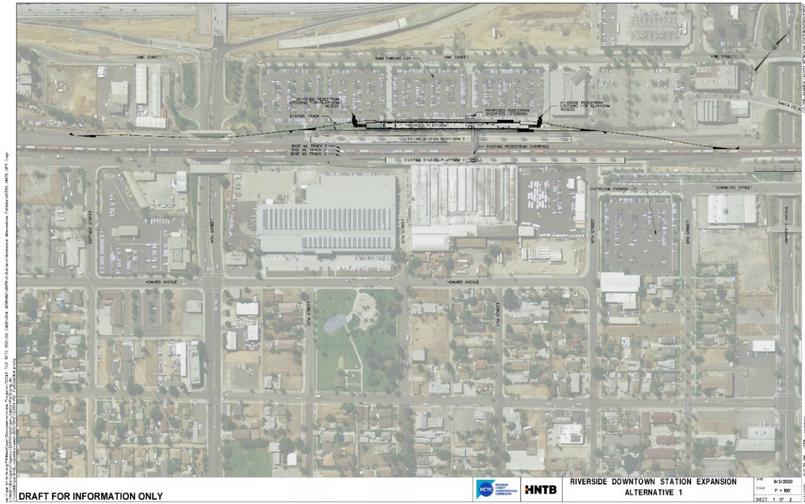
Figure 5-1. Avoidance Alternative 1 New Platform and Tracks on the West Side of the Existing Station
