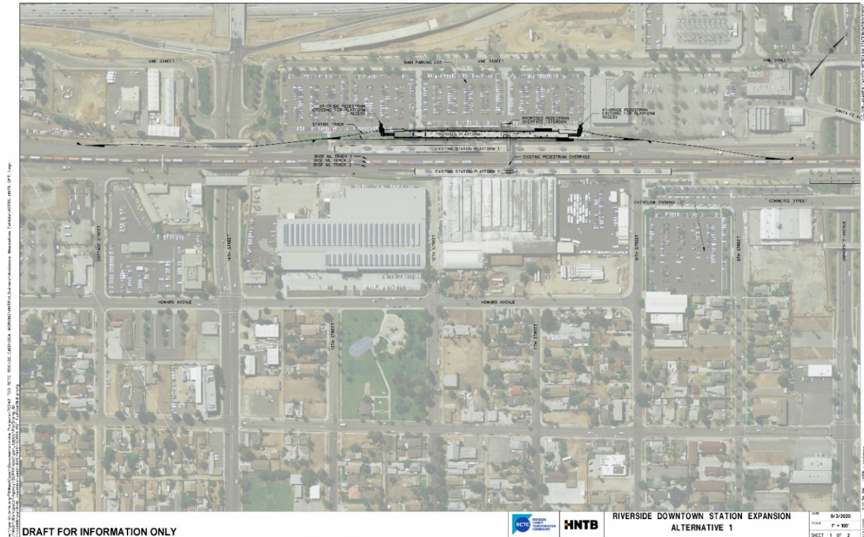
Figure 5-1. Avoidance Alternative 1 New Platform and Tracks on the West Side of the Existing Station
