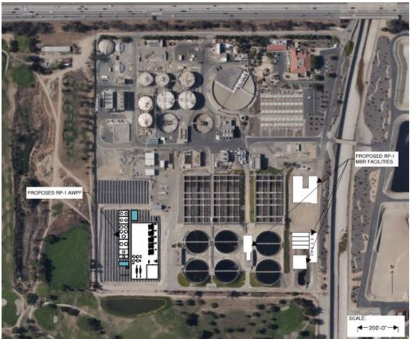
Figure 3-1. RP-1 Site Layout with MBR
