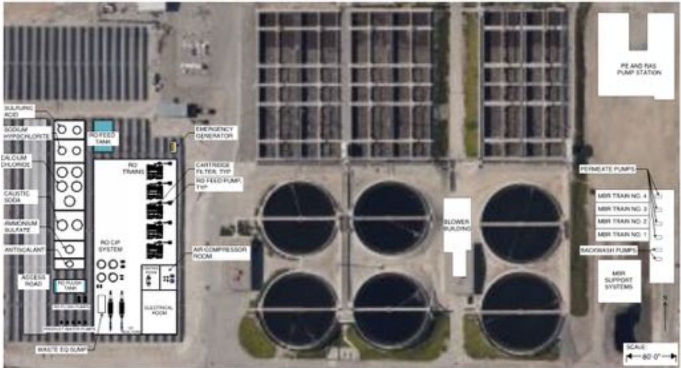
Figure 3-2. RP-1 AWPf and MBR Site Layout
