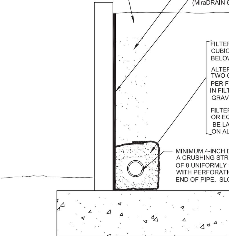
"FILTER MATERIAL" TO MEET FOLLOWING SPECIFICATION OR APPROVED EQUIVALENT: (CONFORMS TO EMA STD. PLAN 323)
