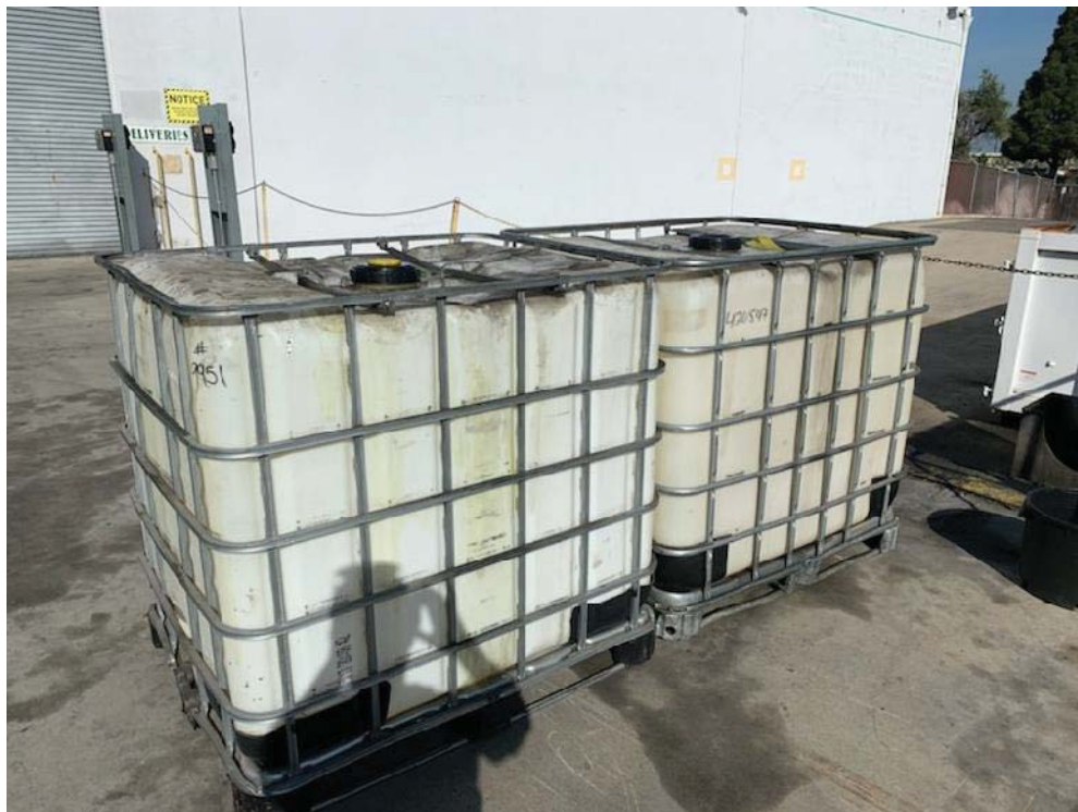
10. Showing plastic containers filled with motor oil. Minor concrete staining below containers
