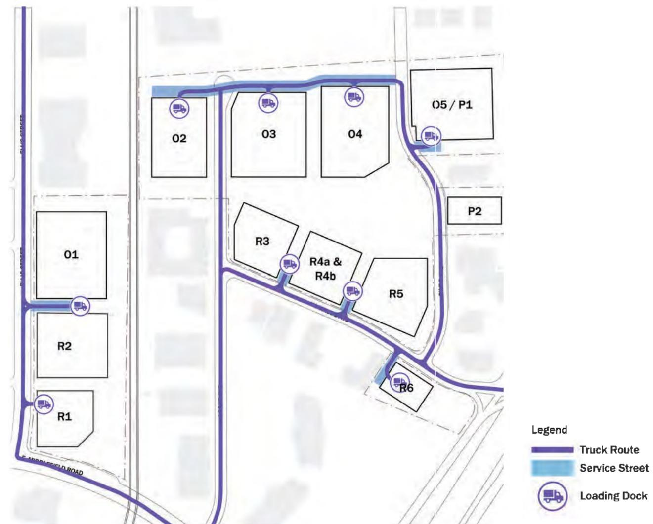
Figure 7.7.2 Truck access and routing
