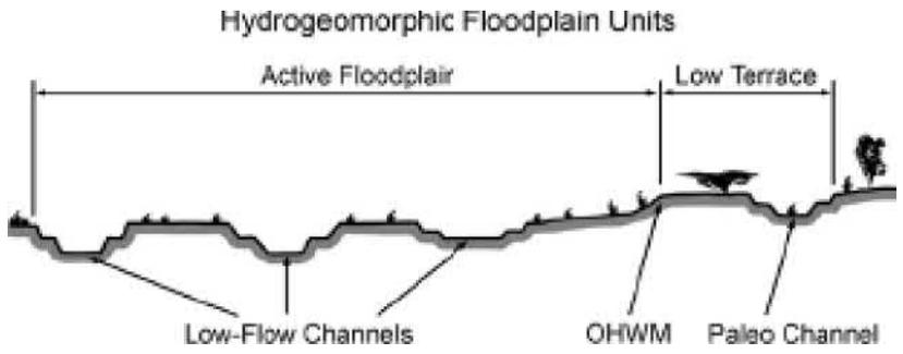
**Procedure for identifying and characterizing the floodplain units to assist in identifying the OHW**
