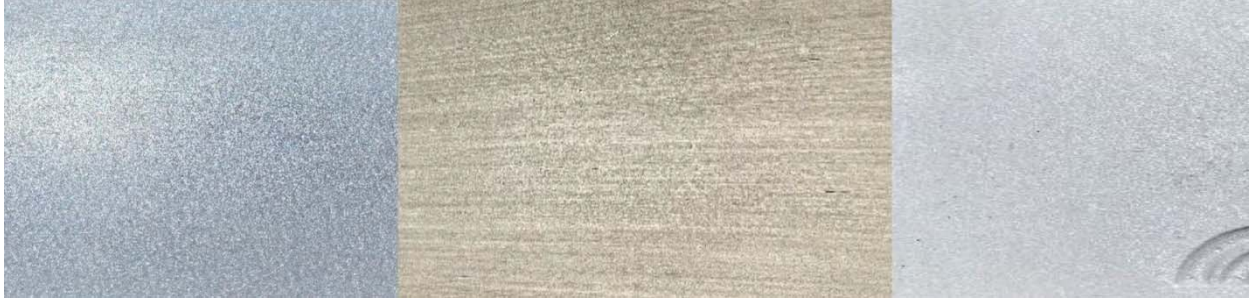
Figure 8. Primary Color and Material Finishes – warm gray pre-weathered Galvalume metal roof, warm gray stain wood body, gray concrete patio material. (Source: IX.1)
