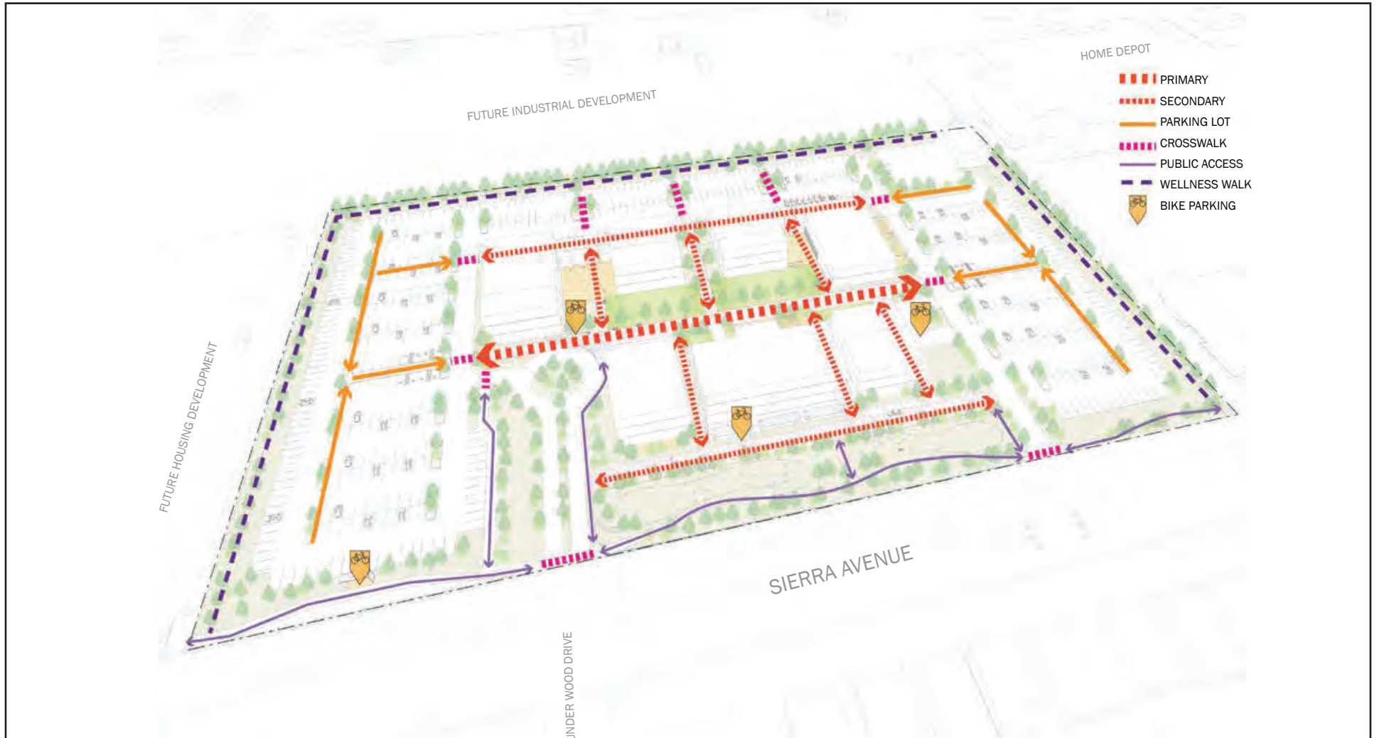
Figure 3-9 - Campus Pedestrian Circulation Plan 3. Project Description
