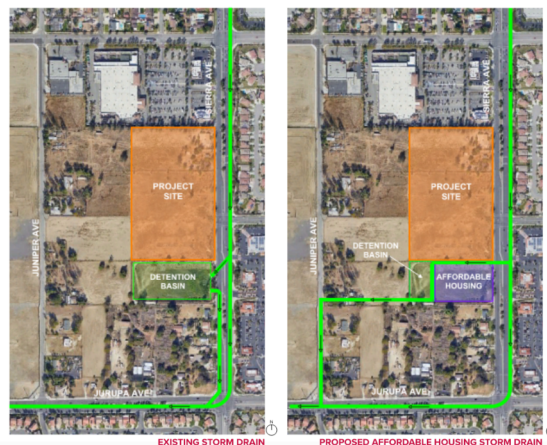
Figure 1: Offsite Existing and Proposed Storm Drain Line
