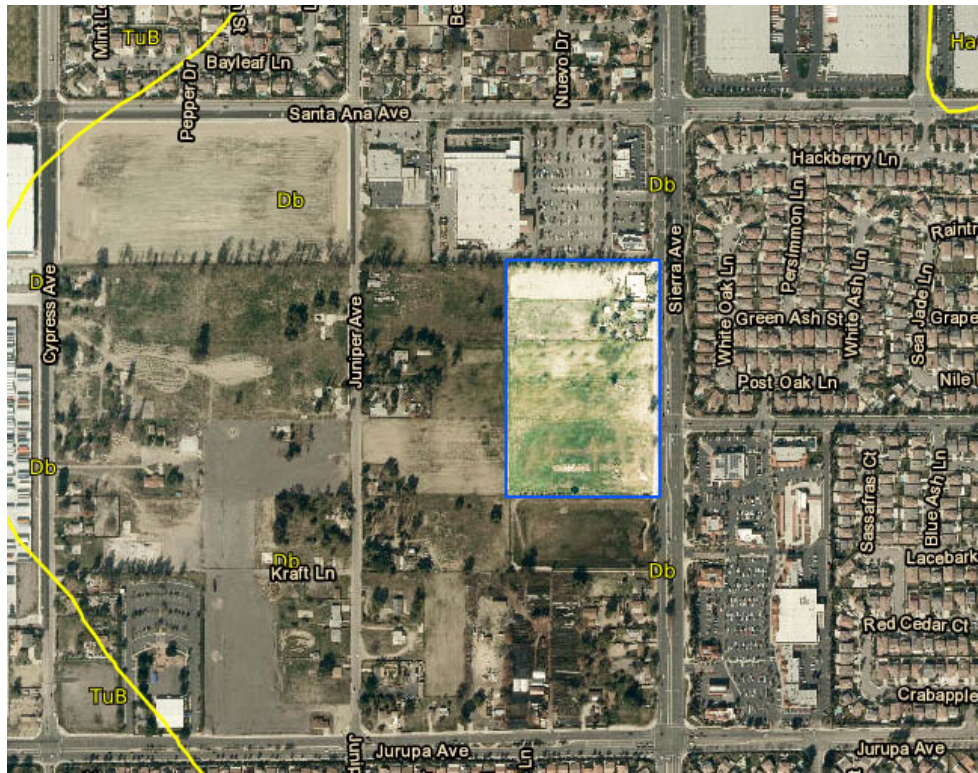
Figure 2. Soils map for the vicinity of the study site (highlighted and outlined in blue): Yellow lines separate soil types: TuB = Tujunga gravelly alluvial soils; Db = Delhi sands.
