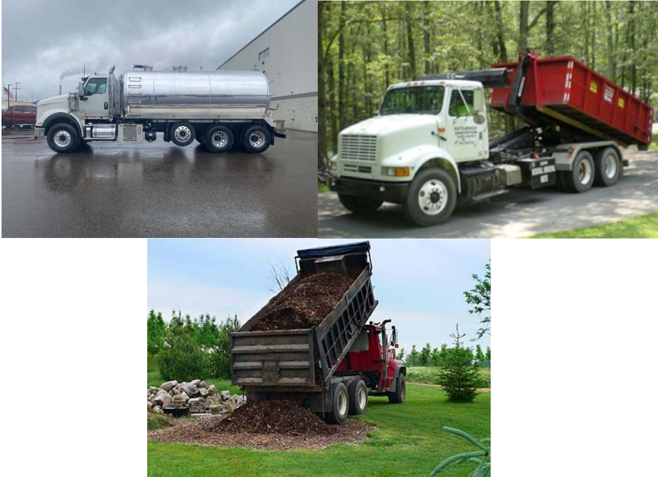
Figure 2: Typical Industrial Waste Trucks – Typical Incoming and Outgoing Liquid Industrial Waste Truck (5,000-Gallon Vacuum Truck; Left); Typical Incoming Solid Industrial Waste Truck (20-40 Cubic Yard Roll Off Truck; Right); and Typical Outgoing Solid Industrial Waste Truck (25-ton Dump Truck; Bottom).
