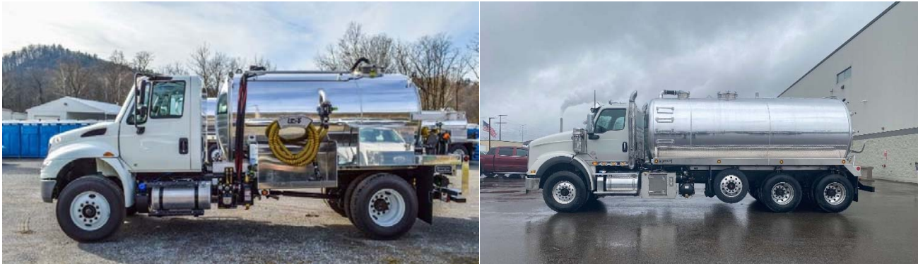
Figure 4: Typical Domestic Waste Trucks – Typical Incoming Liquid Domestic Waste Truck (1,200 to 2,000-Gallon) (Left); and Typical Outgoing Liquid Domestic Waste Truck (6,000-Gallon) (Right).
