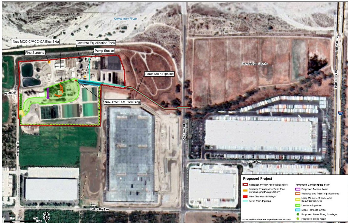
FIGURE 2-3: MODIFICATIONS TO THE EXISTING WWTP
