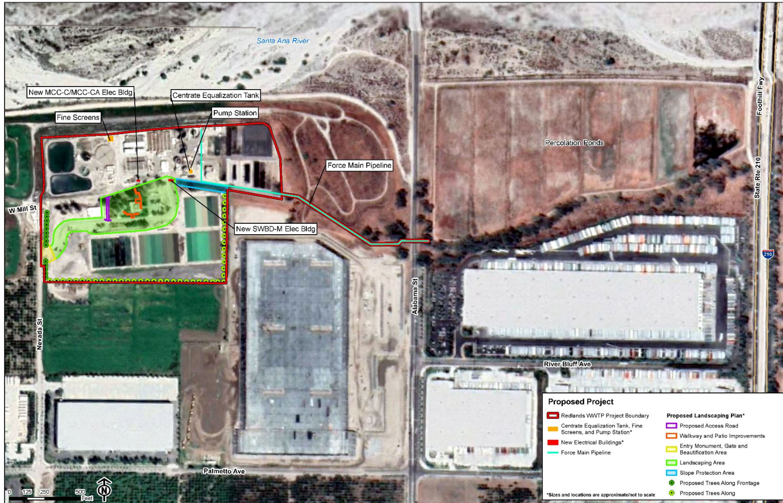
Figure 1. Preliminary Site Layout for Redlands WWTP
