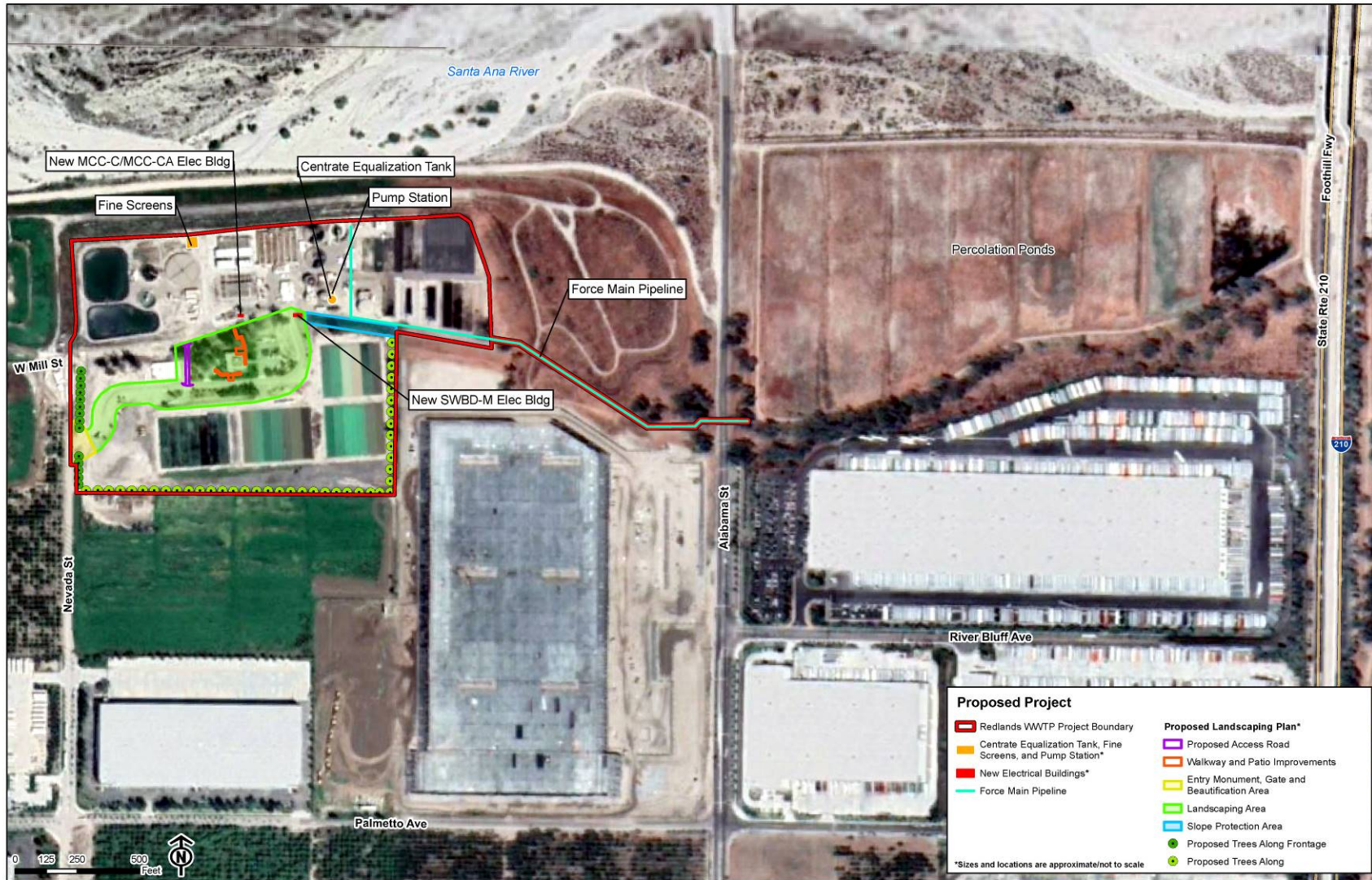
Figure 4. Proposed Modifications to the Existing WWTP
