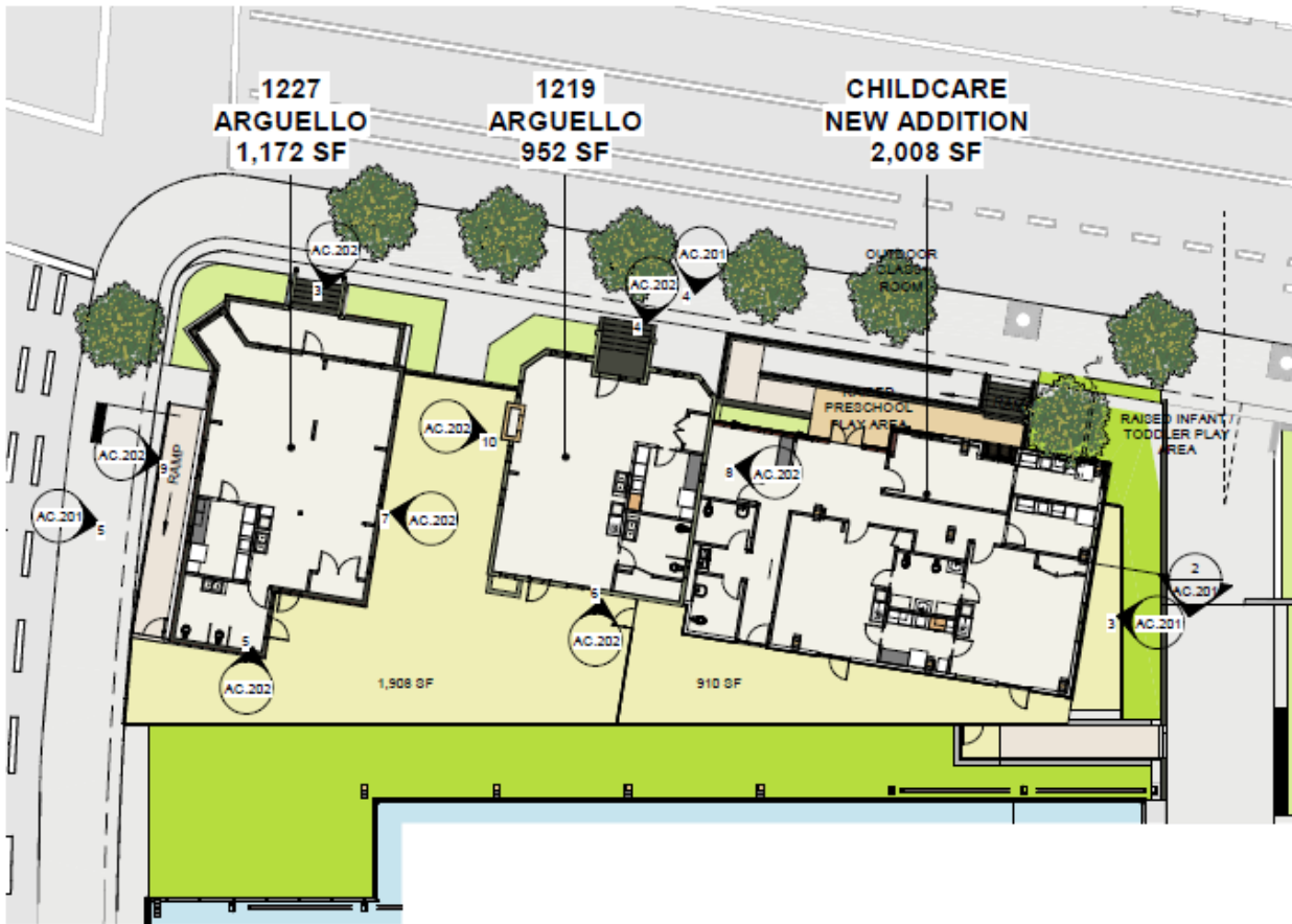
Figure 12. Site plan of rehabilitated 1227 and 1219 Arguello Street for childcare center, with new childcare building abutting the south side of 1219 Arguello Street. Source: DLR Group, "1111-1227 Arguello Street Planning Application" (May 7, 2021), Sheet AC.201.
