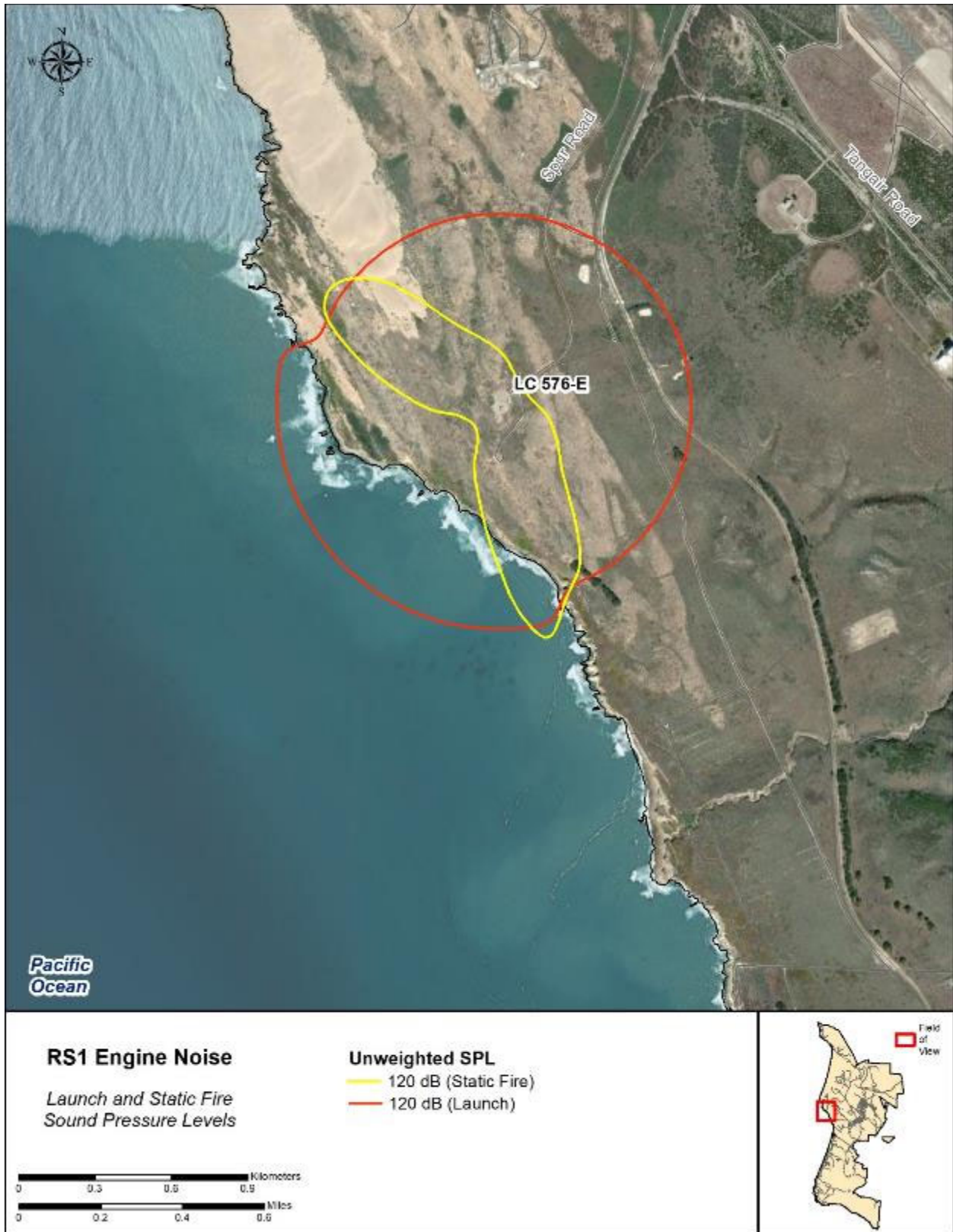
Figure 3.6-1. Launch and static fire unweighted 120 dB sound pressure level contours (Blue Ridge Research and Consulting 2020)
