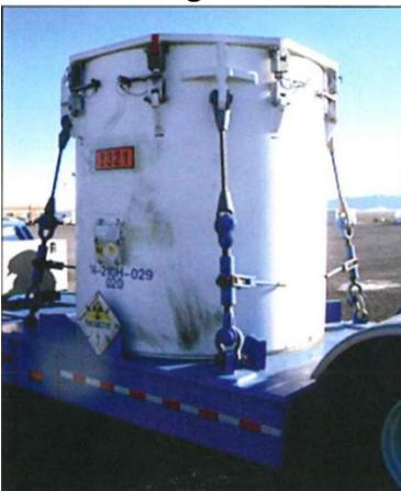
**Figure 2-15. Example of Class B/C Waste Package**
