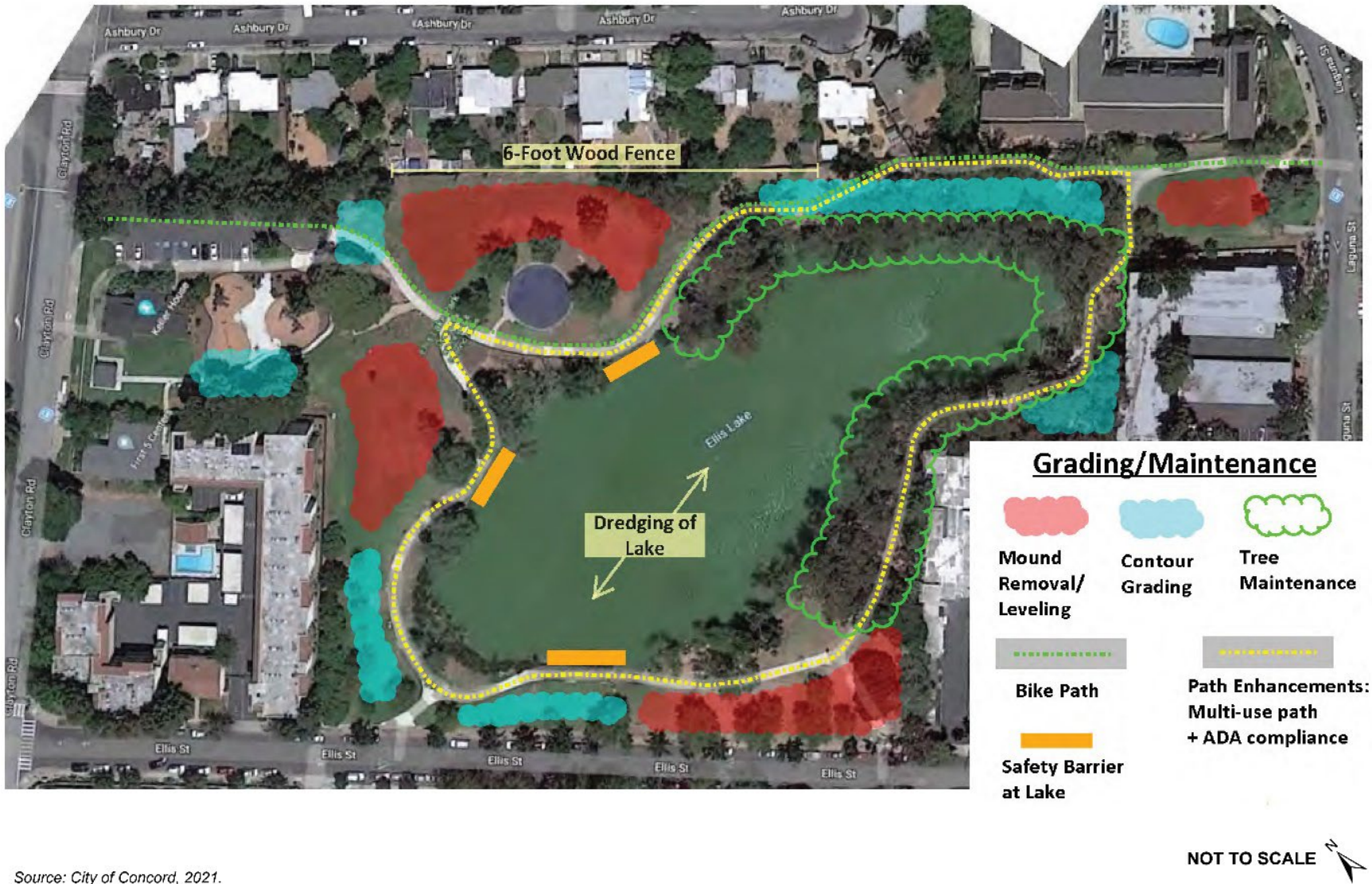
Figure 4 Grading and Maintenance Plan
